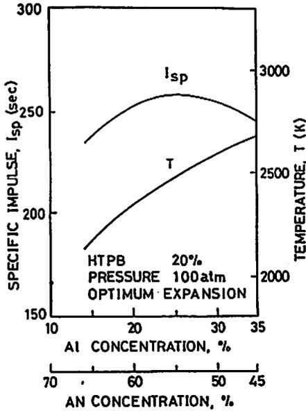
Fig. 1 Variations of specific impulse and flame temperature as a function of Al concentration.
