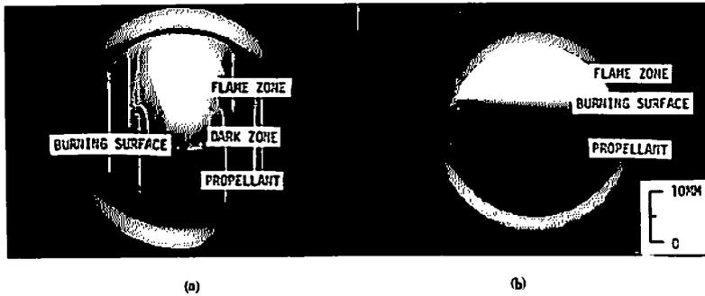
Fig. 10 Photographs of propellant burning without and with crossflow
