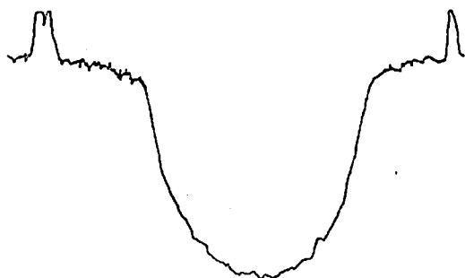
Fig. 5 Film density (1.1mm behind the detonation front)
