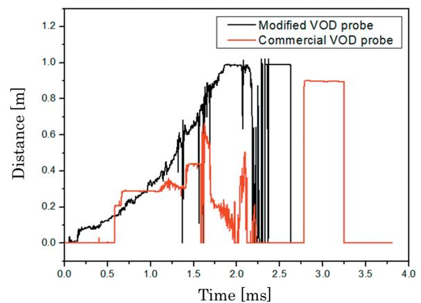
Figure 6 Comparison of VODR profiles with different probe types.
