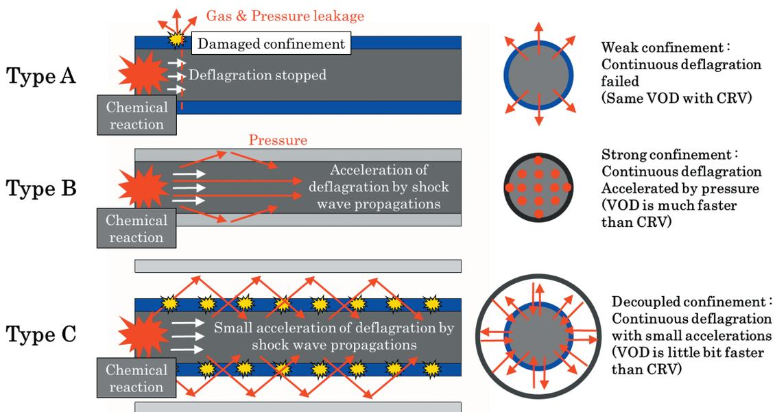
Figure 11 Schematics of continuous deflagration mechanism of thermite reaction agents with different charging states.
