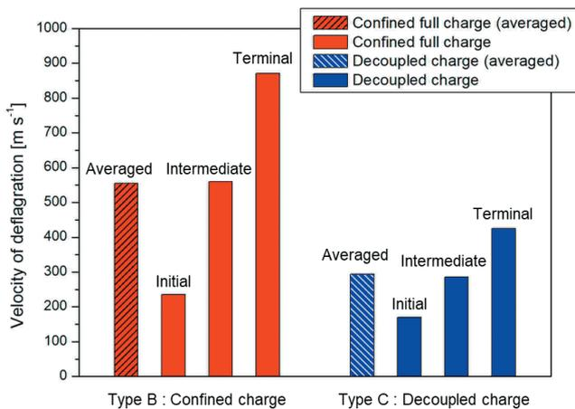
Figure 10 Histogram of VODR comparison between type B and C.
