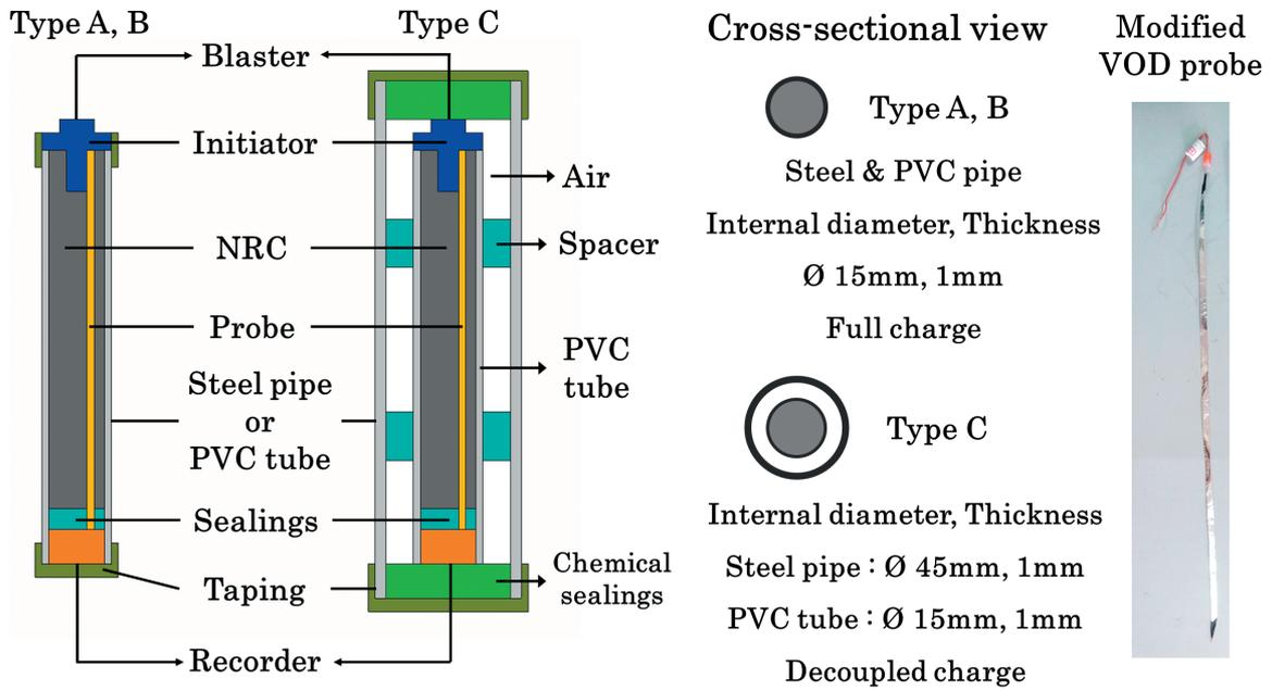
Figure 4 Schematics of VODR measurement system.
