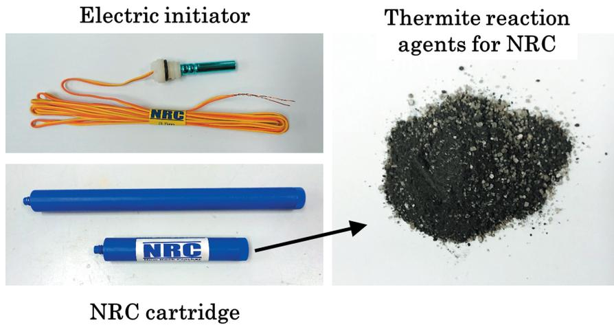
Figure 1 Photographs of NRC and electric initiator.
