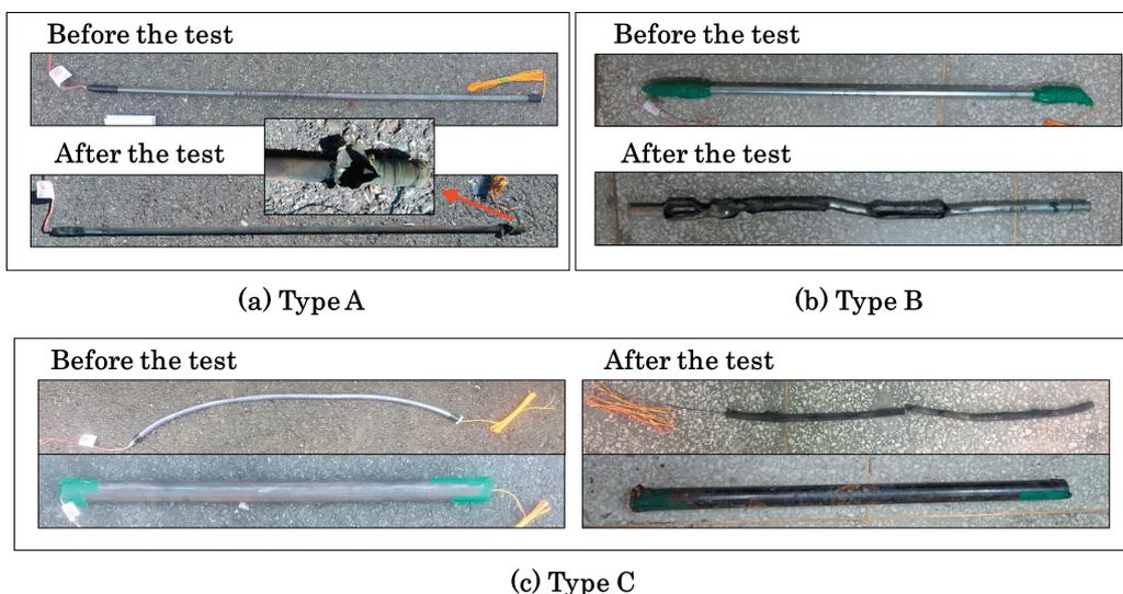
Figure 7 Photographs of charging pipes and tubes; before and after the test.
