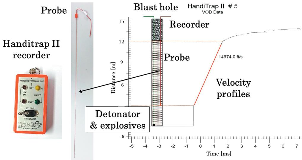
Figure 2 Schematics of typical VOD measurement system.
