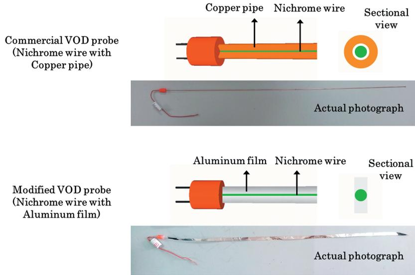
Figure 3 Schematic of different types of VODR probe.
