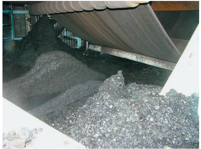
Figure 10 Coal accumulation around transport facilities.
