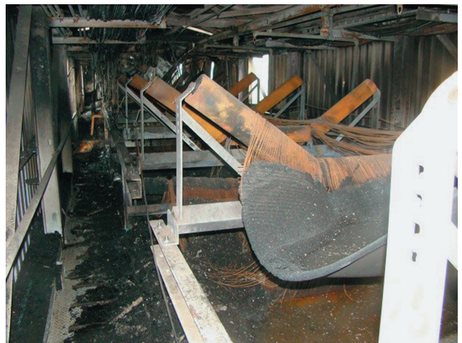
Figure 11 Broken conveyor belt slipped.
