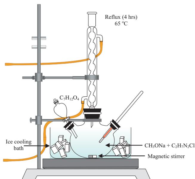
Figure 1 Experimental setup for preparation of 2-methylpyrimidine-4,6-diol.
