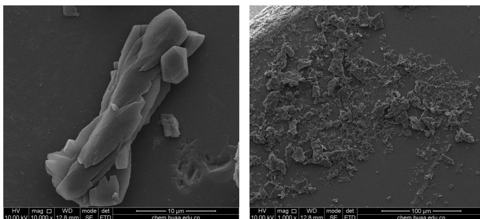
Figure 13 SEM photos of FOX-7 crystals.
