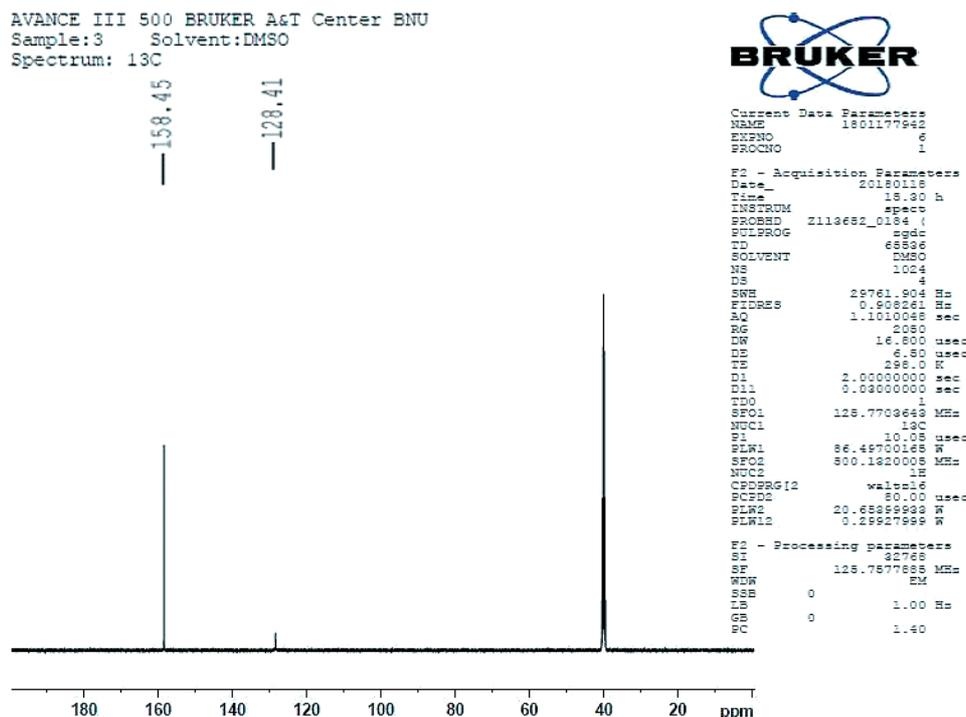
Figure 11  $^{13}\text{C}$  NMR spectrum of FOX-7.
