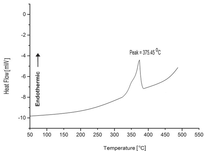
Figure 5 DSC spectrum of 2-methylpyrimidine-4,6-diol.
