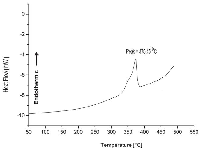
Figure 5 DSC spectrum of 2-methylpyrimidine-4,6-diol.
