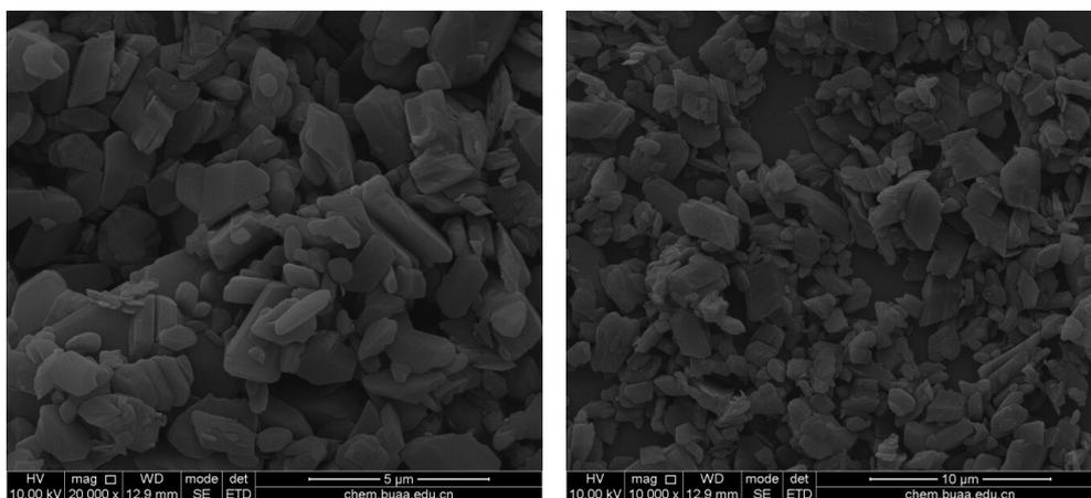
Figure 12 SEM photos of 2-methylpyrimidine-4,6-diol crystals.
