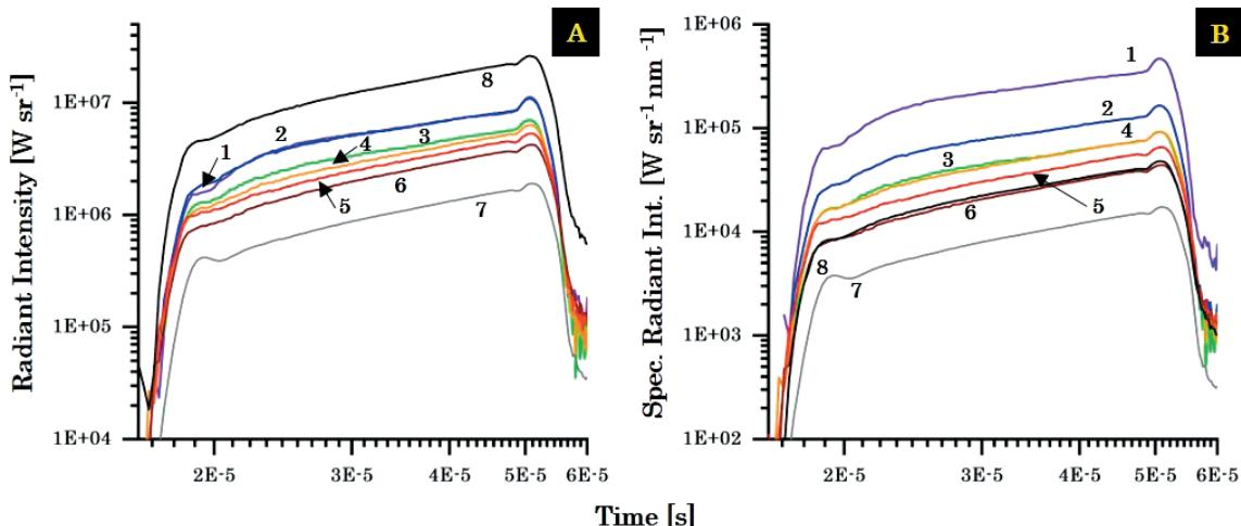
**Figure 6** A 508 mm OD argon flash hemisphere's output in Bands 1–8 is shown in this figure. Note the high spectral temperature indicated in (B) by the peak output occurring in Band 1 (325–350 nm). Also, note the short output duration (approximately 60  $\mu$ s).
