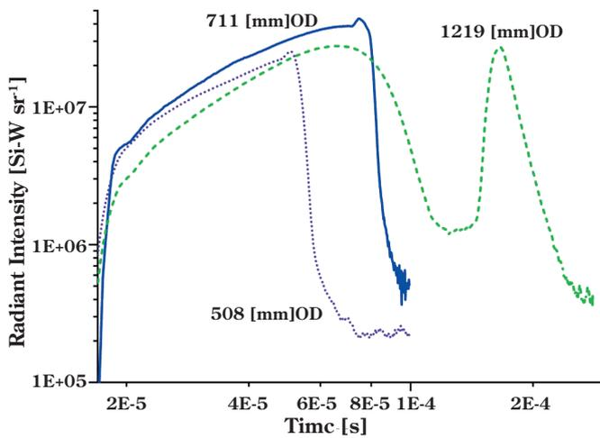
**Figure 8** A comparison of total emission in Band 8 for three hemispheres is shown in this graph. Note that a 711 mm OD hemisphere is the optimal hemisphere diameter for the explosive charge; larger diameters result in shock attenuation leading to decreased emission (1219 mm OD). The sharp rise at late times in the 1219 mm signal is due to shock reflection at the acrylic window's inner surface.
