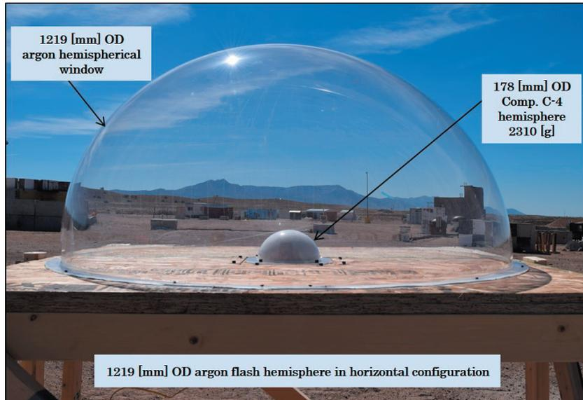
**Figure 3** An argon flash hemisphere consists of an outer acrylic shell (1219 mm OD × 4.76 mm thick) mounted to a wooden base. A hemisphere of Composition C-4 (178 mm OD) is mounted concentrically to the wooden base; argon gas fills cavity through ports in the base (not shown).
