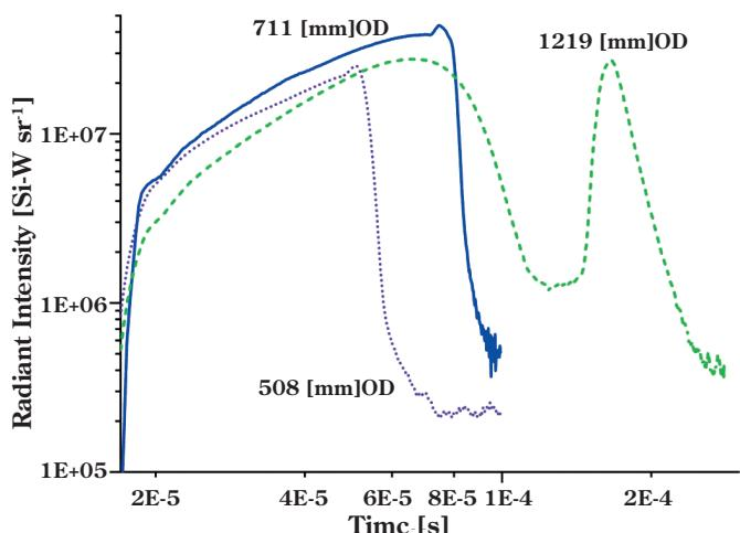
**Figure 8** A comparison of total emission in Band 8 for three hemispheres is shown in this graph. Note that a 711 mm OD hemisphere is the optimal hemisphere diameter for the explosive charge; larger diameters result in shock attenuation leading to decreased emission (1219 mm OD). The sharp rise at late times in the 1219 mm signal is due to shock reflection at the acrylic window's inner surface.
