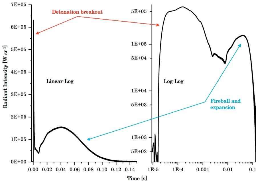
**Figure 1** A sample broadband (Si-band) optical signature for 4.5 kg of Composition C-4 is shown in these images. Data are identical; however, they are plotted on linear-log and log-log plots. A short and intense light emission is observed at early times followed by a sharp decrease and then a second emission increase (fireball).
