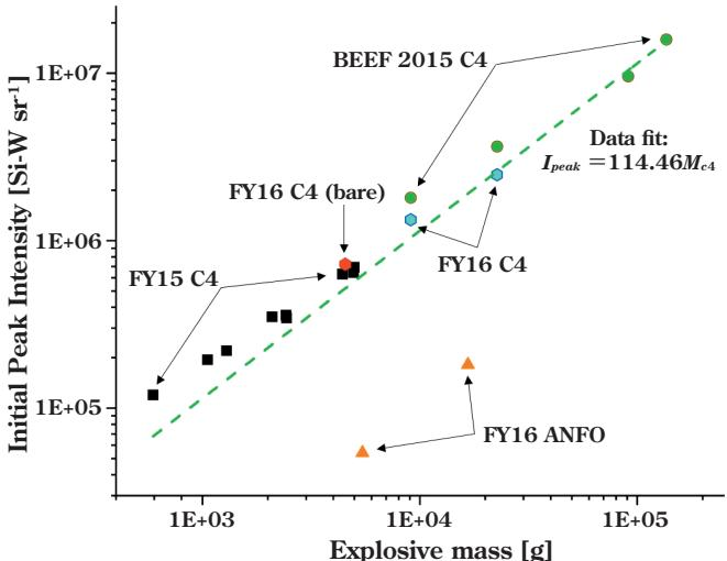
**Figure 9** This plot summarizes the peak intensity in Band 8 (Si-band) from Composition C-4 charges. The peak intensity correlates well with charge mass over several decades of mass. The correlation fit only considers Composition C-4 explosive tests; two ANFO (lower detonation pressure) tests are also shown for comparison.
