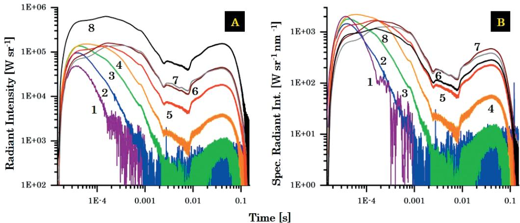
**Figure 5** Total and spectral intensities in Bands 1–8 of a representative Composition C-4 charge are shown in this figure. Numbers next to each line indicate the optical band. Spectral measurements (B) are normalized to the FWHM of each band.
