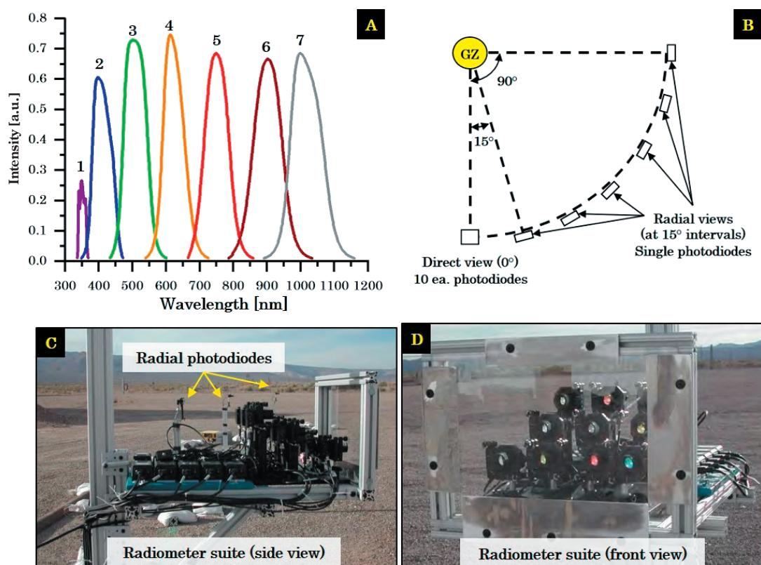
**Figure 4** Details of the radiometer setup are summarized in this image: A) band coverage in visible and NIR regimes; B) radial layout (overhead view) of photodiodes in addition to direct view setup ("GZ" = Ground Zero); C) side view of direct and radial photodiodes, and D) front view of direct photodiodes. Note: two additional photodiodes were mounted in the direct view setup; their data are not reported.
