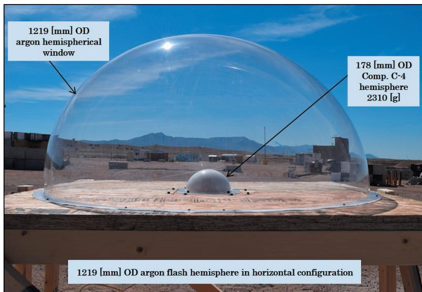
**Figure 3** An argon flash hemisphere consists of an outer acrylic shell (1219 mm OD  $\times$  4.76 mm thick) mounted to a wooden base. A hemisphere of Composition C-4 (178 mm OD) is mounted concentrically to the wooden base; argon gas fills cavity through ports in the base (not shown).
