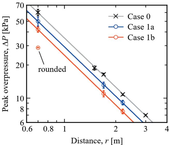
Figure 3 Peak overpressure distribution.
