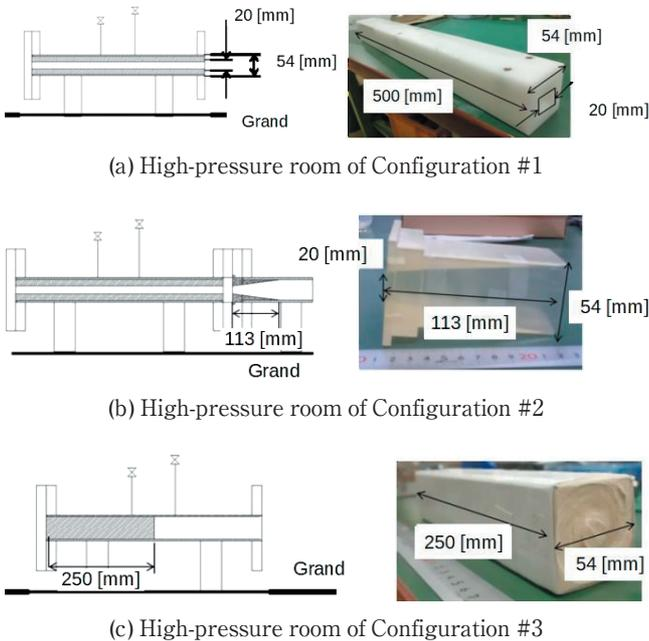
**Figure 3** Modifications of the high-pressure room of 5×5ST to generate shock waves followed by negative pressure.
