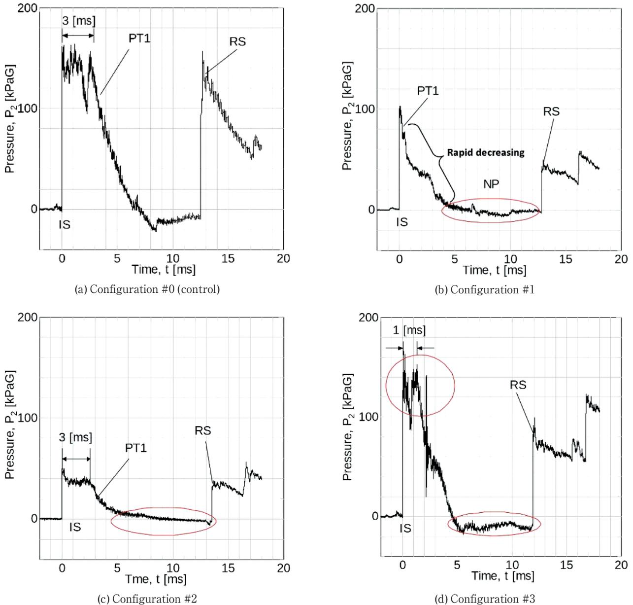
Figure 4 Pressure histories at PT1 after arrival of the incident shock.
