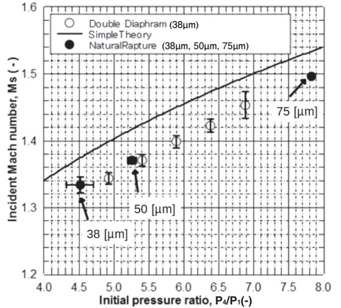
Figure 2 The characteristics of 5×5ST on the parametric plane of the initial pressure ratio  $P_4/P_1$  and the incident shock Mach number  $M_s$ . The values shown in the figure represent the thicknesses of the used diaphragms.
