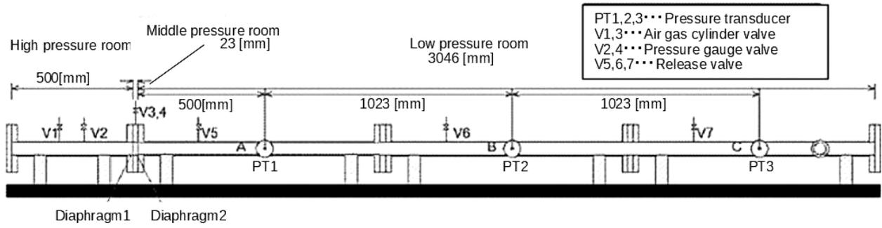
Figure 1 Schematic diagram of a 50-mm-by-50-mm shock tube.
