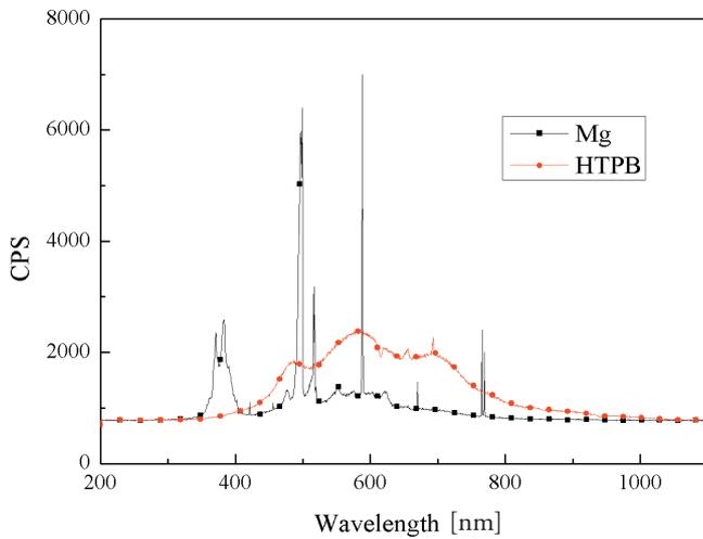
**Figure 7** Spectra of HTPB and magnesium under atmospheric pressure.
