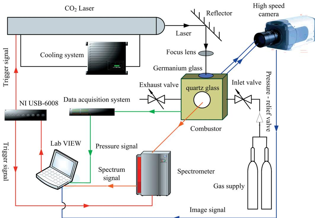
Figure 2 The schematic drawing of the experimental facility.
