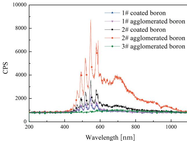
Figure10 Spectra of coated boron and agglomerated boron.
