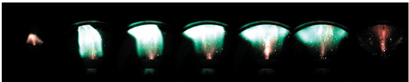
Figure 5 High-speed camera images of 2# agglomerated boron.
