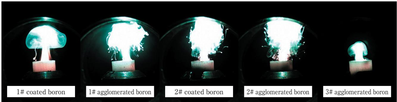
Figure 12 The combustion photos under 2 MPa at air atmosphere.
