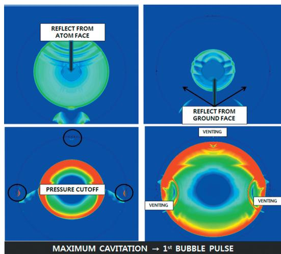
Figure 8 Pressure behavior of central charge ( $d : 200$  mm).
