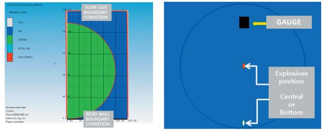
(a) Boundary condition (b) Pressure gauge and explosives position
