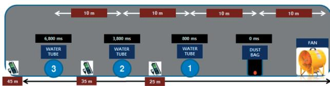
(c) Time difference for explosion (considering wind speed attenuation)
