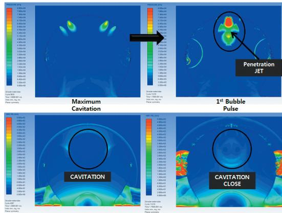
Figure 7 Pressure behavior of bottom charge ( $d : 200$  mm).
