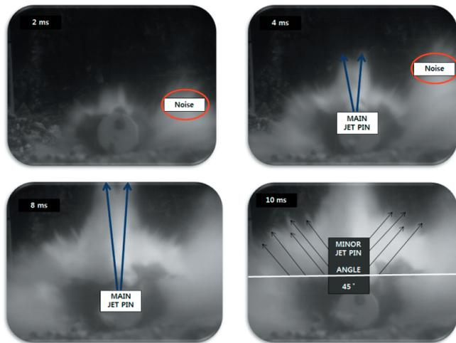
**Figure 4** Jet pin movement after explosion for bottom charge.
