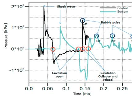
**Figure 6** Time history of shock wave and gas bubble pressure pulse (Water tube, AUTODYN).
