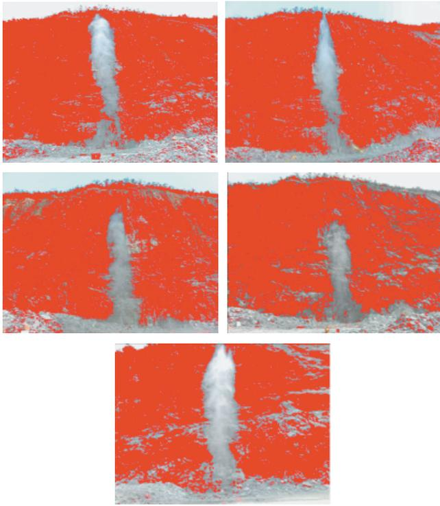
**Figure 3** Cross-sectional form of mist diffusion (bottom charge).
