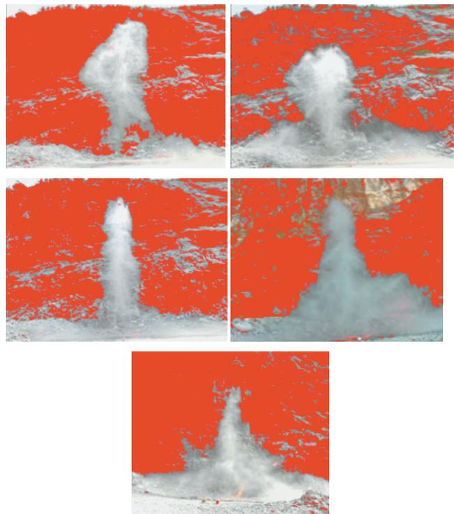
**Figure 2** Cross-sectional form of mist diffusion (central charge).
