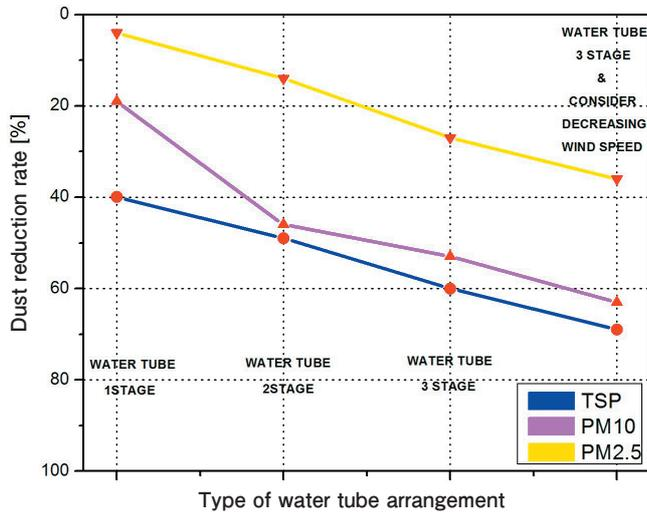
Figure 11 Dust reduction rate of water tube per experimental case.
