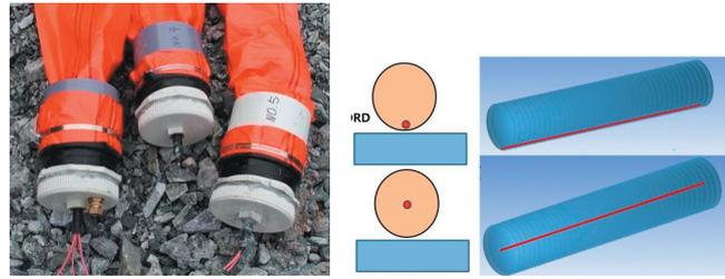
**Figure 1** Form of water tube and explosion position of charge (bottom charge & central charge).
