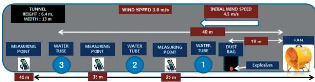
(a) Position of water tube and dust measuring instrument
