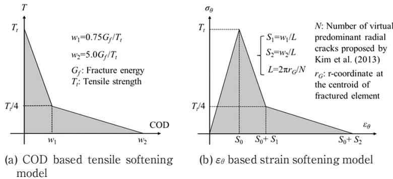
Figure 5 Model for non-linear crack opening behavior.
