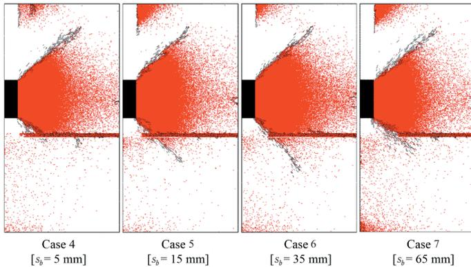
**Figure 10** Influence of spacing between steel plate and charge hole,  $S_b$ , on fracture pattern [ $P_0 = 100$  MPa,  $t_0 = 50$   $\mu$ s].
