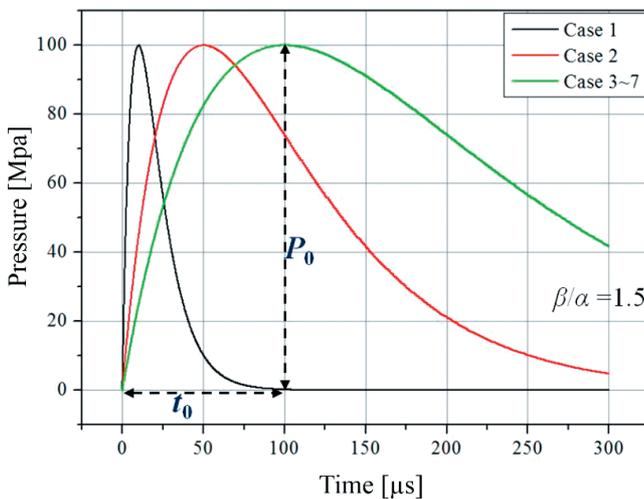
**Figure 7** Pressure-time curve for applied pressure waveform for Table 2.
