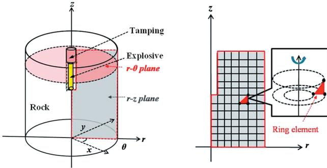
(a) 3-D cylindrical charge model. (b) Axisymmetric FEM model
