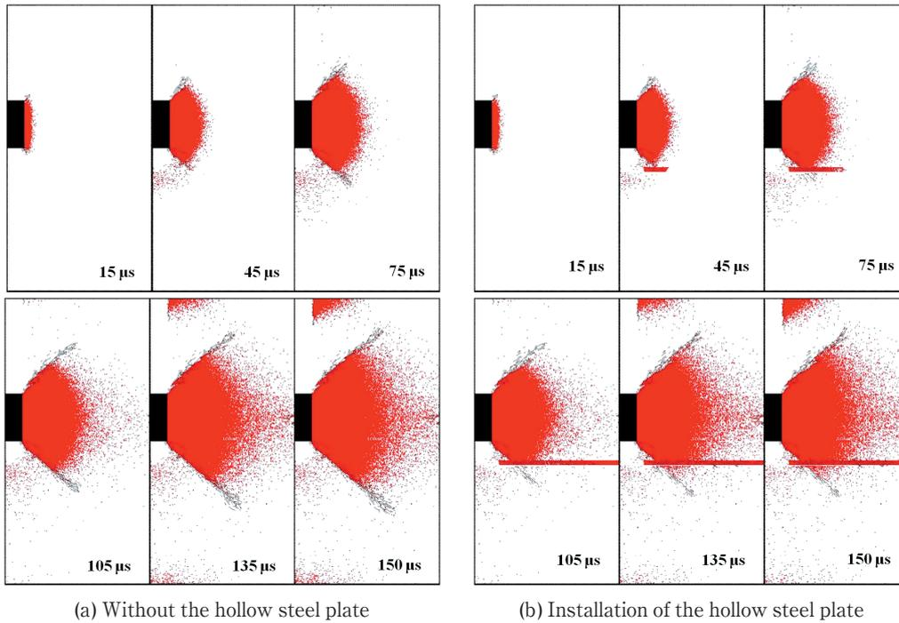
**Figure 8** Result of fracture process in with/without the hollow steel plate.
