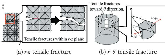
Figure 4 Axisymmetric FEM model.
