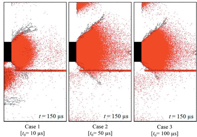
**Figure 9** Influence of rise time,  $t_0$ , on the resultant fracture pattern [ $P_0 = 100 \text{ MPa}$ ,  $S_b = 90 \text{ mm}$ ].
