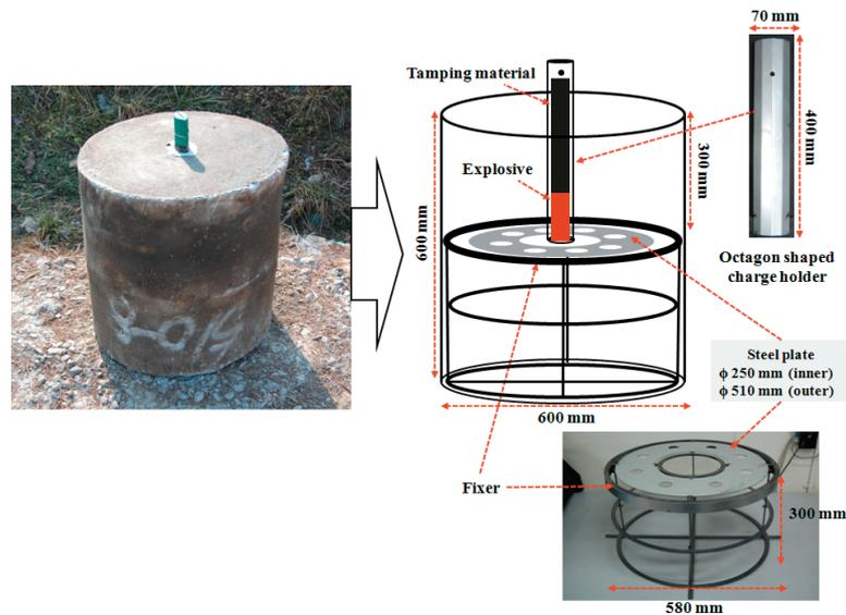
Figure 1 Description of the specimen used in the blasting experiments.
