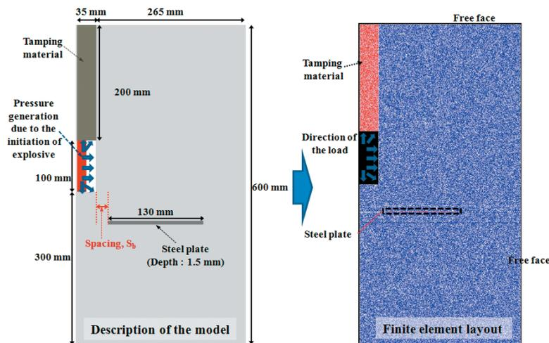
Figure 6 Description of the finite element mesh having a hollow steel plate.
