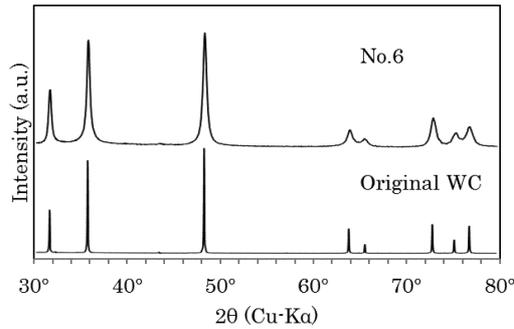
**Figure 6** XRD pattern (Cu K $\alpha$ ) taken from upper surface of No.6 and original WC powder.
