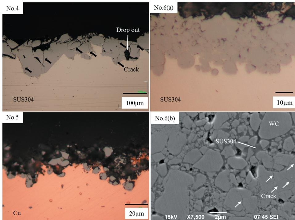
**Figure 7** Cross-sectional optical (No.4–6) and SEM (No.6) image of recovered driver plate.
