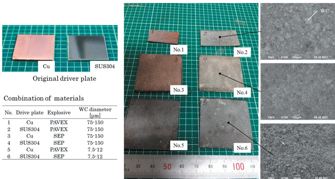
Figure 5 External appearance and the surface SEM images of the recovered driver plates.
