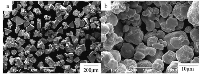
Figure 2 SEM image of WC powder particles (a: coarse particle, 75–150 $\mu\text{m}$ , b: fine particle 7.5–12 $\mu\text{m}$ ).
