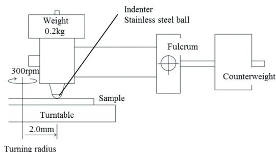
Figure 8 Schematic diagram of wear test apparatus.
