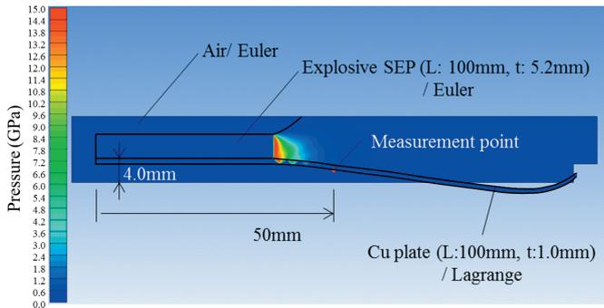
Figure 3 2-dimensional analysis model and flight process by explosive detonation.
