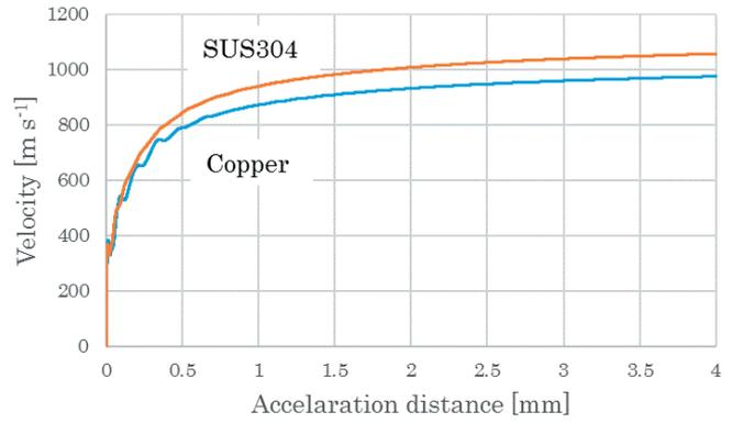
Figure 4 Analysis result of driver plate velocity at each acceleration distance.
