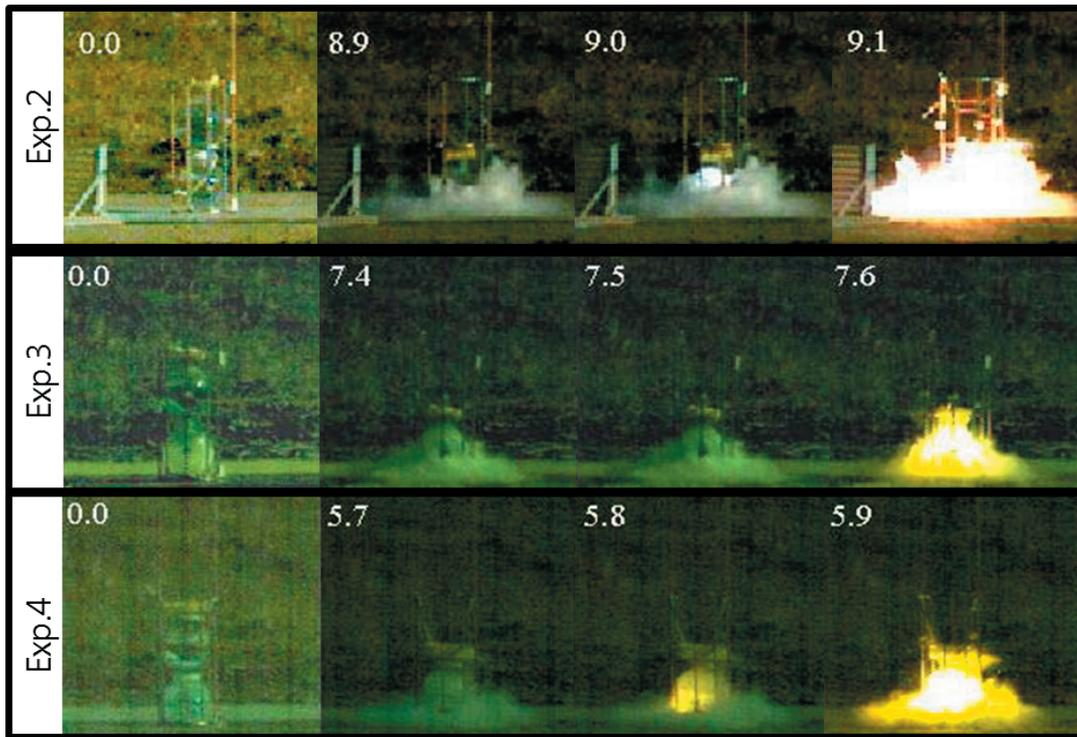
Figure 2 Framing images obtained with a high-speed camera during the collision (unit : ms)
