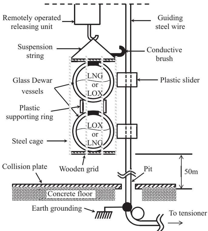
Figure 1 Experimental setup for drop test.
