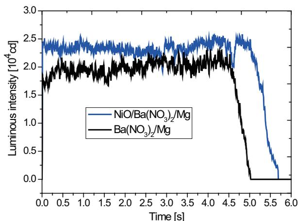
**Figure 4** The luminous intensity *vs* time curves for  $\text{Ba}(\text{NO}_3)_2/\text{Mg}$  and  $\text{NiO}/\text{Ba}(\text{NO}_3)_2/\text{Mg}$ .
