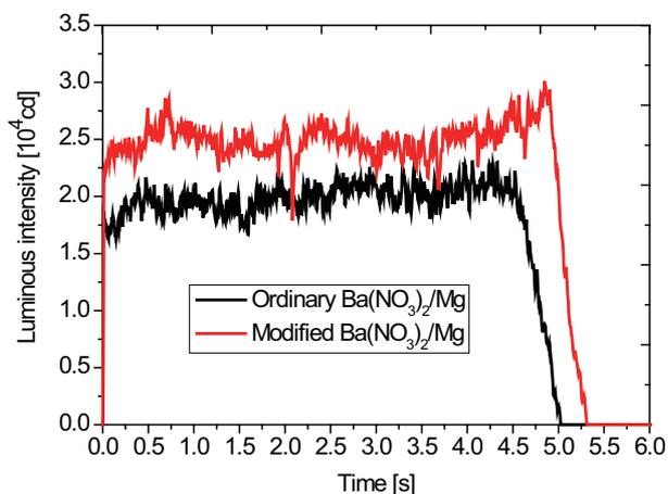
**Figure 3** The luminous intensity *vs* time curves for  $\text{Ba}(\text{NO}_3)_2/\text{Mg}$  and modified  $\text{Ba}(\text{NO}_3)_2/\text{Mg}$ .
