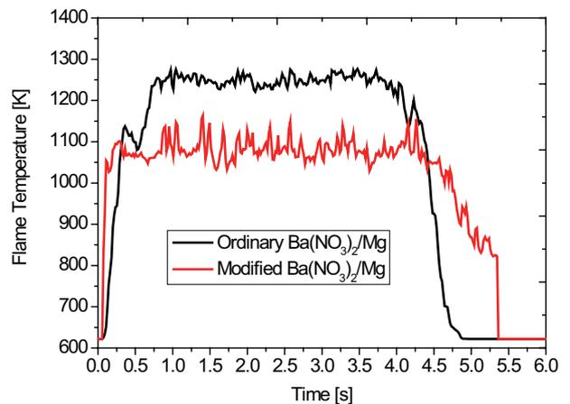
**Figure 2** The flame temperature *vs* time curves.**Table 2** Average optical combustion characteristics for ordinary Ba(NO<sub>3</sub>)<sub>2</sub>/Mg and modified Ba(NO<sub>3</sub>)<sub>2</sub>/Mg.
