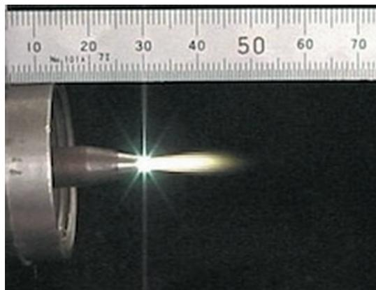
Figure 2 Photo of O<sub>2</sub> plasma jet at  $P_{in} = 100$  W with  $Q_f = 1$  NL min<sup>-1</sup>.
