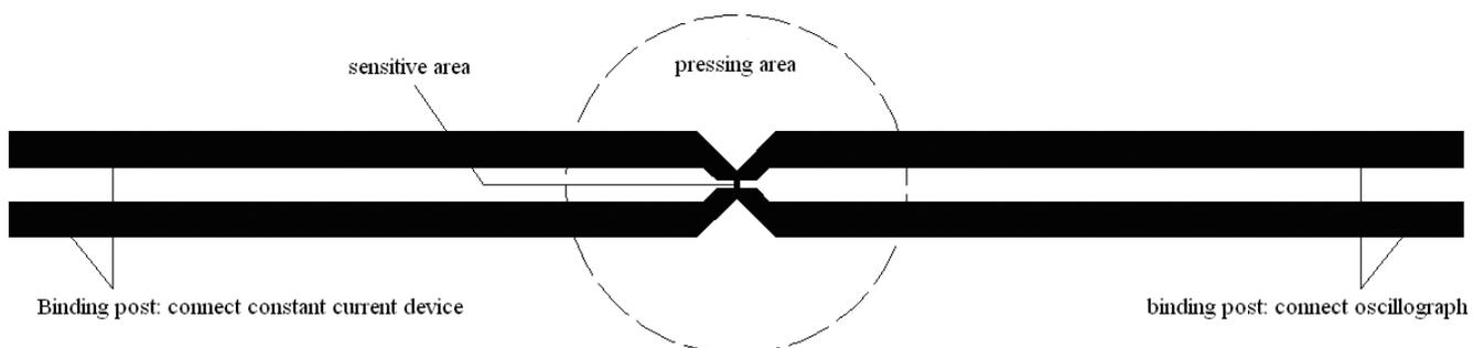
Figure 3 Structural sketch of micro manganin piezoresistive sensor.
