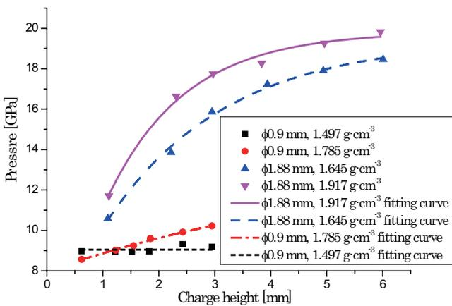
**Figure 5** Relation between detonation pressure and charge heights of PBXN-5 with micro charge.
