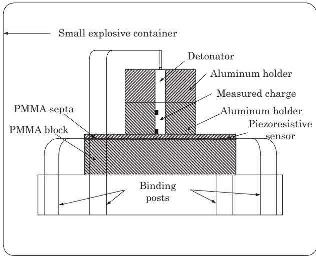
Figure 1 The schematic diagram of micro charge detonation pressure measurement system.
