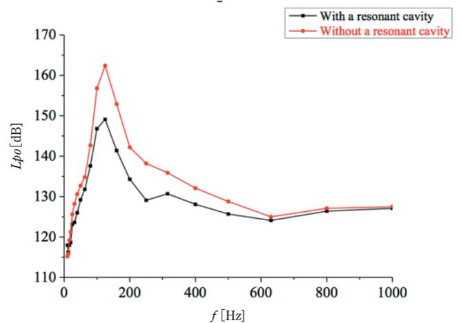
Figure 3 Frequency of a feedback cavity similar to a Hartmann acoustic generator on the SPL of underwater pyrotechnic combustion ( $D_c = 10 \text{ mm}$ ,  $D_r = 12.5 \text{ mm}$ , the distance between the cavity charge nozzle and the feedback cavity was  $10 \text{ mm}$ ).
