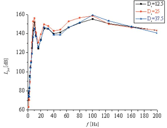
**Figure 7** Effect of feedback cavity diameter on the SPL of underwater pyrotechnic combustion
