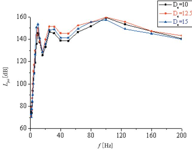
**Figure 6** Effect of nozzle diameter on the SPL of underwater pyrotechnic combustion.
