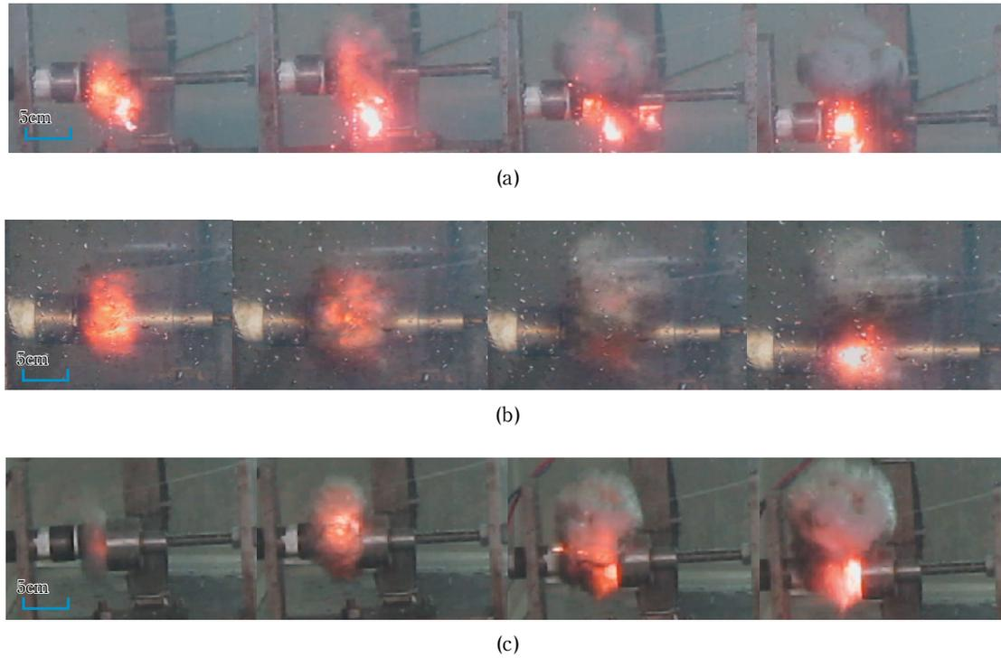
**Figure 8** Pattern of pyrotechnic combustion bubbles with a feedback cavity diameter of (a) 12.5, (b) 25 and (c) 37.5 mm (feedback cavity on the right and charge cavity on the left,  $D_c = 10$  mm, the distance between the cavity charge nozzle and the feedback cavity was 25 mm).
