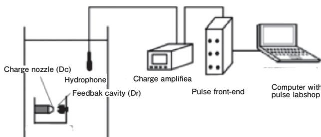
Figure 2 Schematic diagram of the underwater pyrotechnic combustion test.
