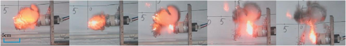
**Figure 4** The bubble pattern of underwater pyrotechnic combustion without a feedback cavity (charge cavity on the left).
