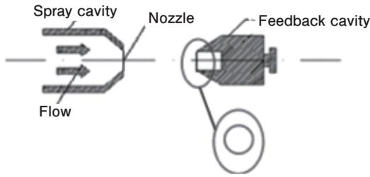
Figure 1 Schematic diagram of a Hartmann acoustic generator.
