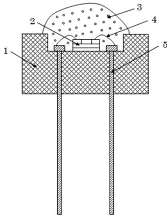
**Figure 1** Schematic diagram of SCB initiator.
