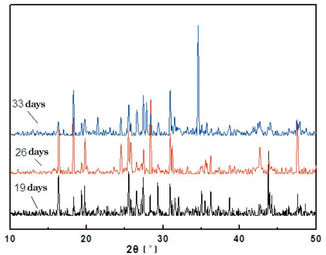
Figure 10 XRD patterns comparison of 19, 26, 33 days aged ignition powder.
