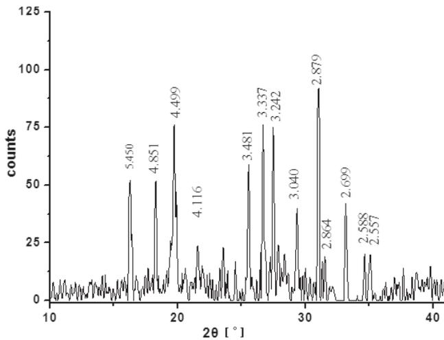
Figure 7 XRD pattern of none aged ignition powder.
