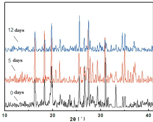
Figure 8 XRD patterns comparison of 0, 5, 12 days aged ignition powder.
