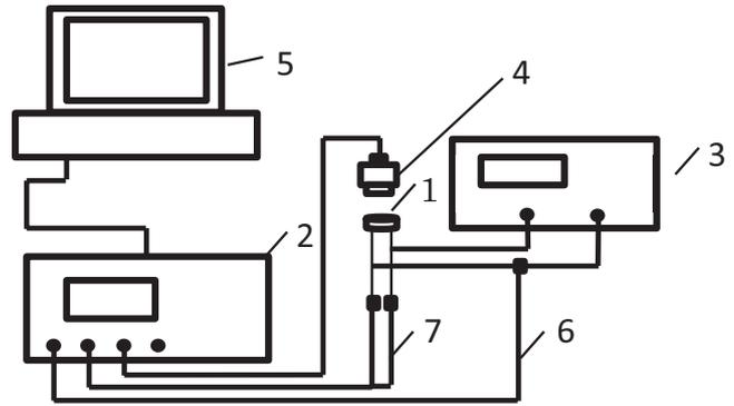
**Figure 2** Schematic diagram of the SCB electro-exploding experimental setup.
