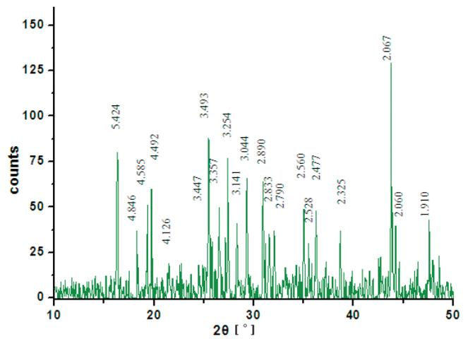
Figure 9 XRD pattern of 19 days aged ignition powder.
