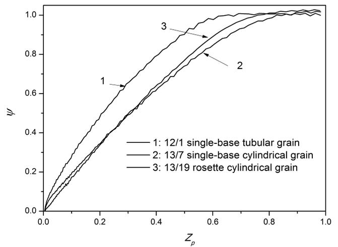
**Figure 2**  $\Psi-Z_p$  curve calculated by experimental pressure-apparent burning rate model. (1): 12/1 single-base tubular grain; (2): 13/7 single-base cylindrical grain; (3) 13/19 rosette single-base cylindrical propellant
