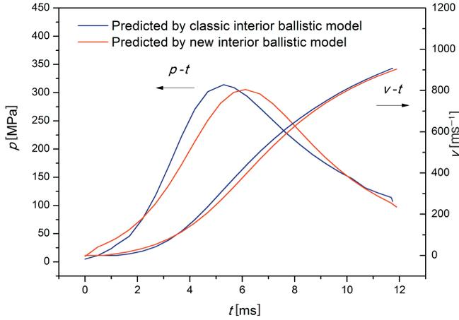
**Figure 3** Mean pressure and projectile velocity vs. time curves as predicted by classic interior ballistic and new interior ballistic method based on experimental-apparent burning rate model.
