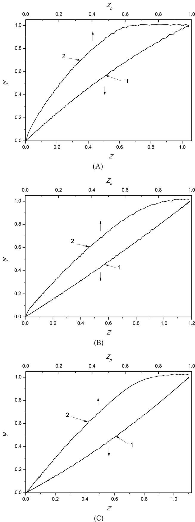
**Figure 1** Comparison of  $\Psi-Z_p$  curve of three kinds of propellants. (A) 12/1 single-base propellant (B) 13/7 single-base propellant (C) 13/9 single-base propellant calculated by two kinds of different models: 1-Traditional form function method; 2-experimental pressure-apparent burning rate model.
