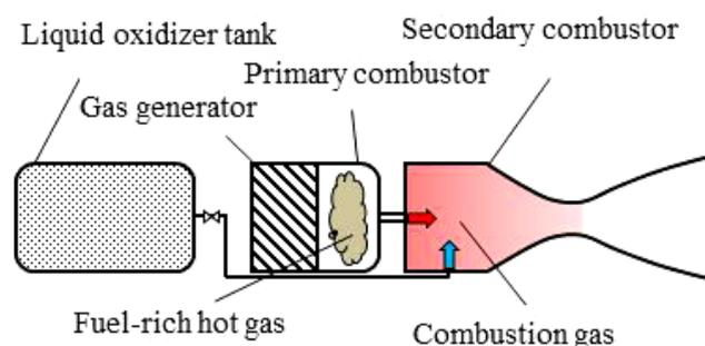
Figure 1 Structure of the gas hybrid rocket.
