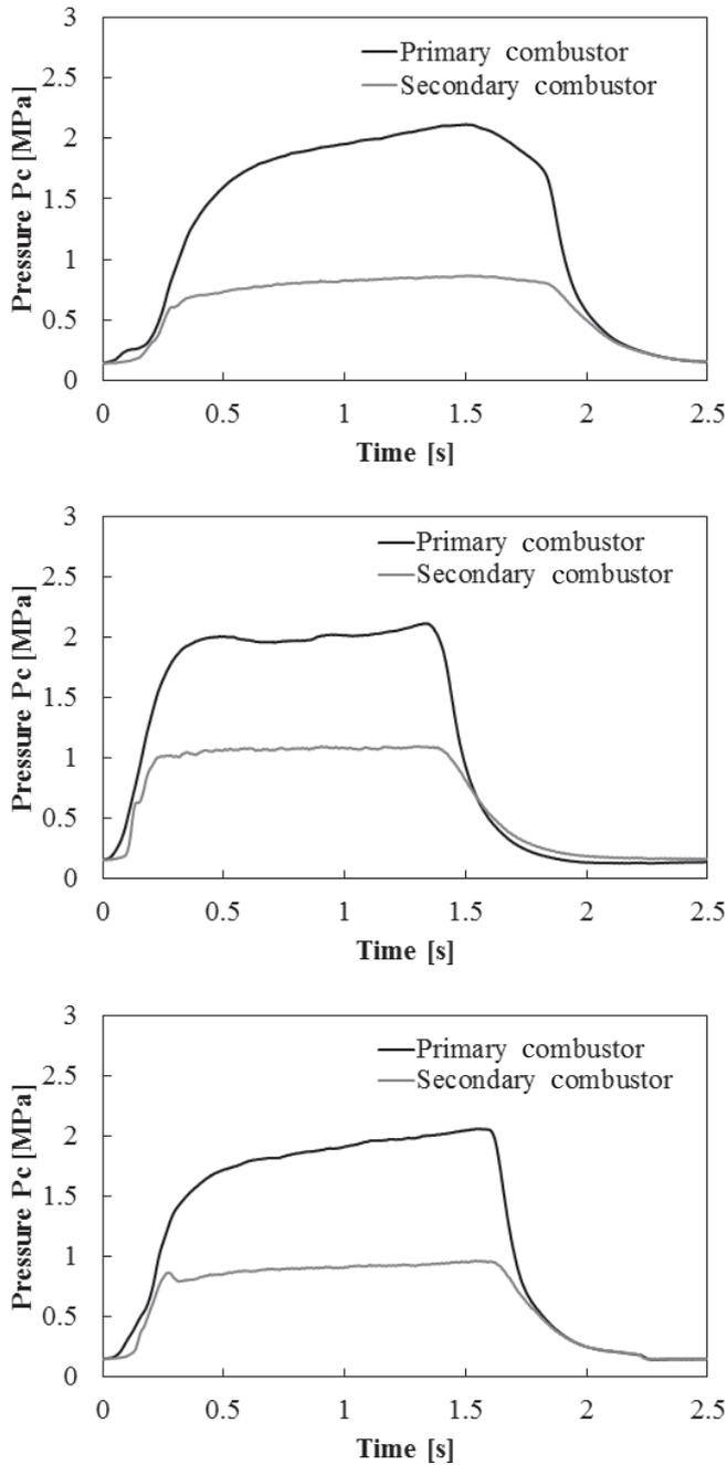
**Figure 6** Pressure histories of the gas hybrid rocket chamber: (a) GAP/AP, (b) GAP/AP/Zr, and (c) GAP/AP/Mg.
