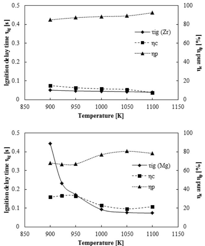
**Figure 5** Relation between the electric furnace temperature and ignition delay time or the ratio of  $\tau_c$  to  $\tau_p$  to the ignition delay time at 0.1 MPa: (a) zirconium 45  $\mu\text{m}$  and (b) magnesium 45  $\mu\text{m}$ .
