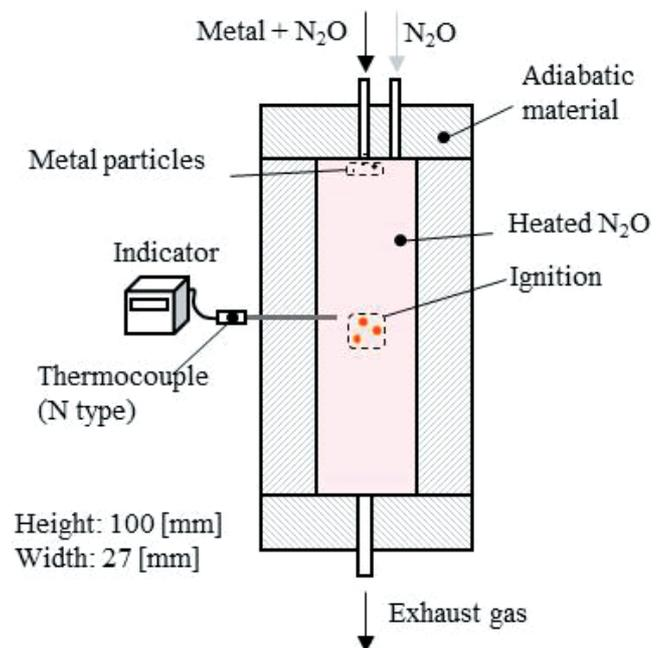
Figure 3 Electric furnace.
