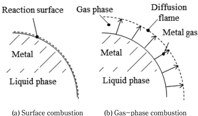
Figure 2 Combustion types of metal particles.
