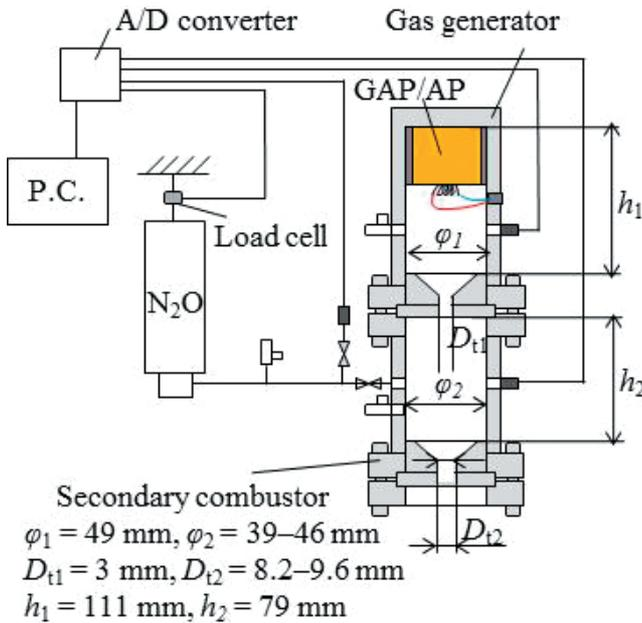
**Figure 4** Experimental apparatus of the gas hybrid rocket.
