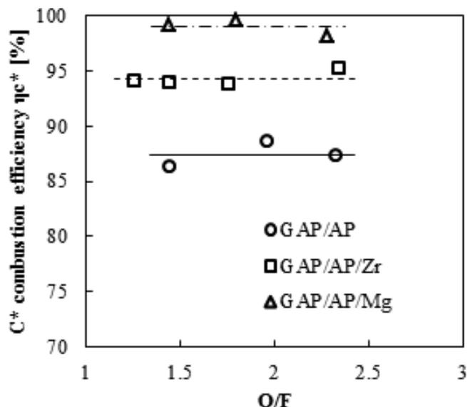
Figure 8 Relation between O/F (N<sub>2</sub>O/fuel) and C\* combustion efficiency.
