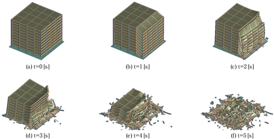
**Figure 5** Collapse behavior (entire collapse) of SL6\_H3\_10S model as per time.
