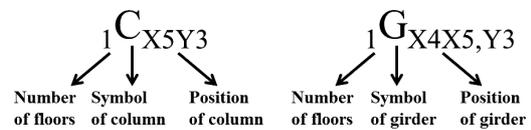
The target columns in each analysis model were 5 column elements ( $1C_{X5Y1}$ ,  $1C_{X5Y2}$ ,  $1C_{X5Y3}$ ,  $1C_{X5Y4}$ ,  $1C_{X5Y5}$ ) in the X5 row on the first floor as shown in Figure 3, and these column elements were removed simultaneously for 0.01 second using the IER (Immaculate Element Method) technique.
