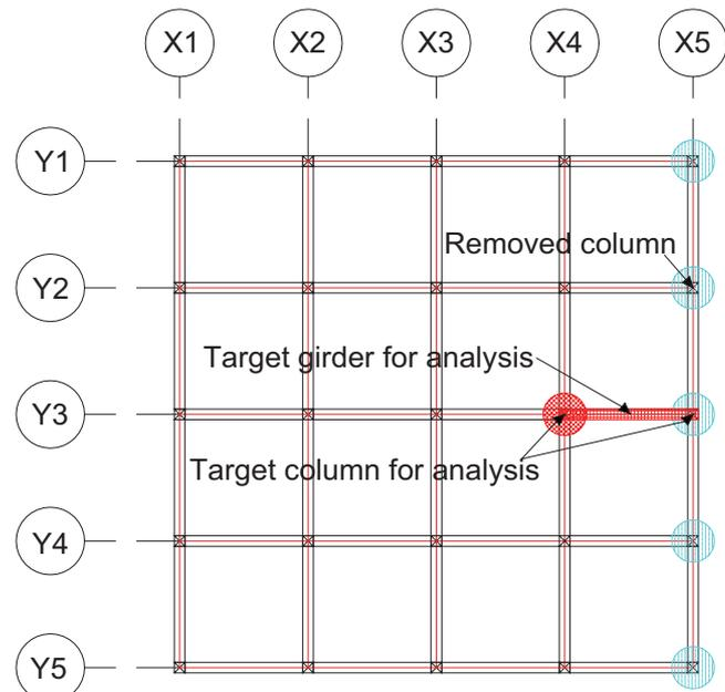
**Figure 3** Position of target columns for removal and the position of target column and girder for analysis.
