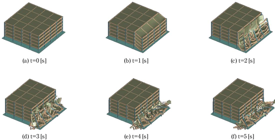
**Figure 4** Collapse behavior (partial collapse) of SL6\_H3\_5S model as per time.
