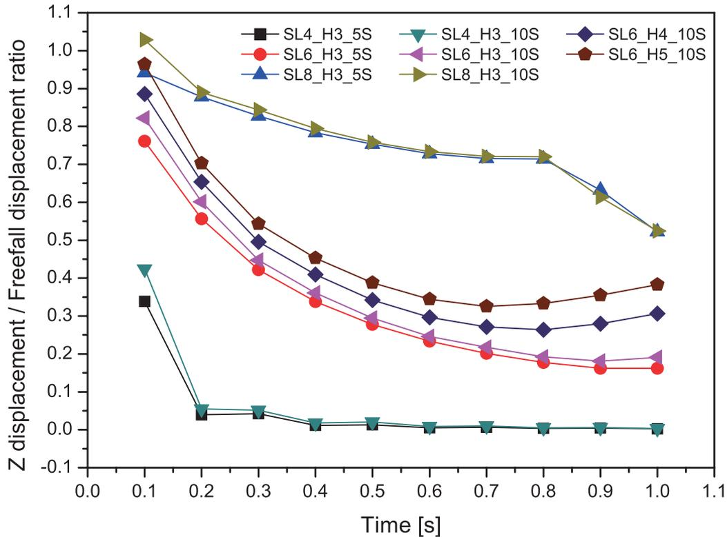
Figure 6 Comparison of ratio between vertical displacement and free fall displacement as per time according to each condition.
