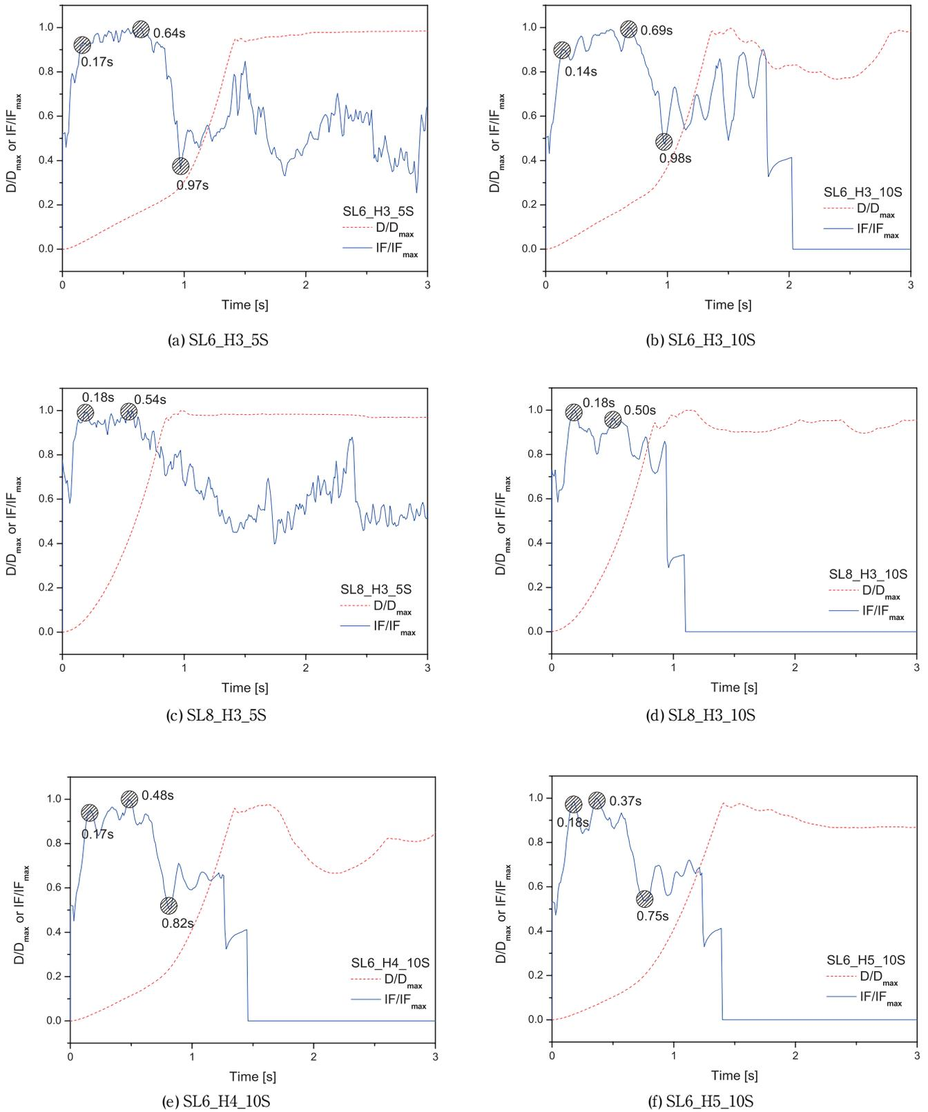
**Figure 7** Comparison between vertical displacement ratio and vertical internal force ratio as per time according to each condition.
