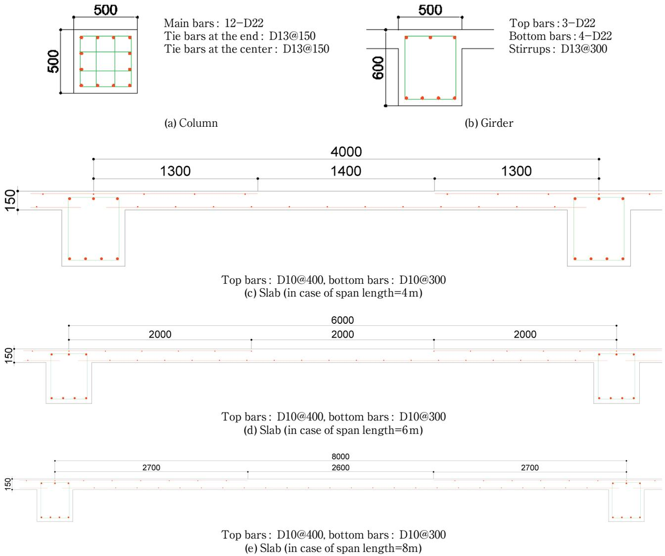
Figure 1 Dimensions of concrete members and reinforcing bar arrangement drawing (unit : mm).
