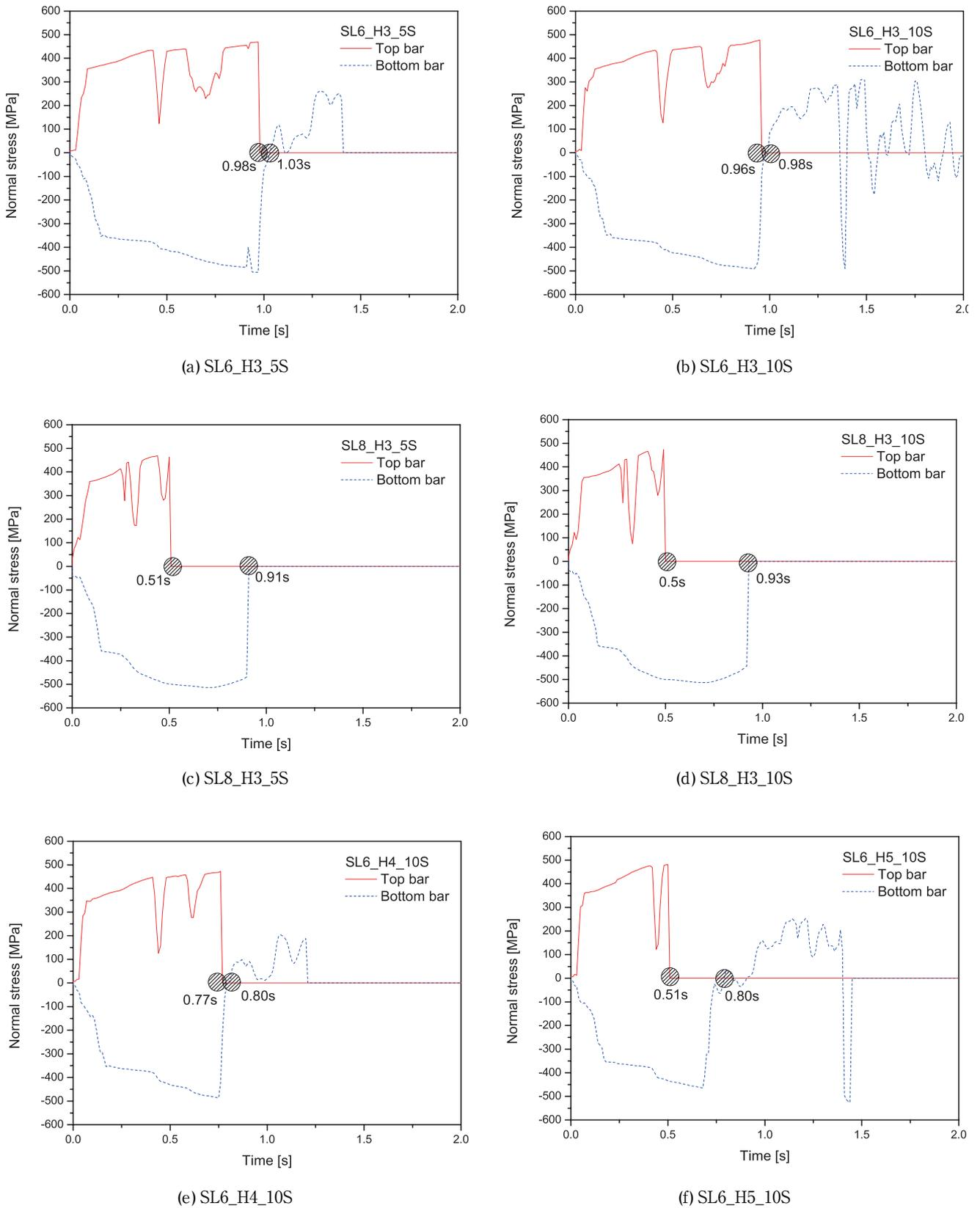
**Figure 8** Comparison of normal stress between top bar and bottom bar as per time according to each condition.
