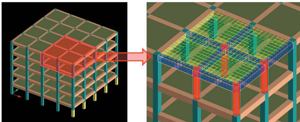
Figure 2 Arrangement status of reinforcing bar in SL4\_H3\_5S model.
