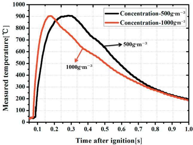
Figure10 Measured temperature profiles of the combustion zone at two concentrations.
