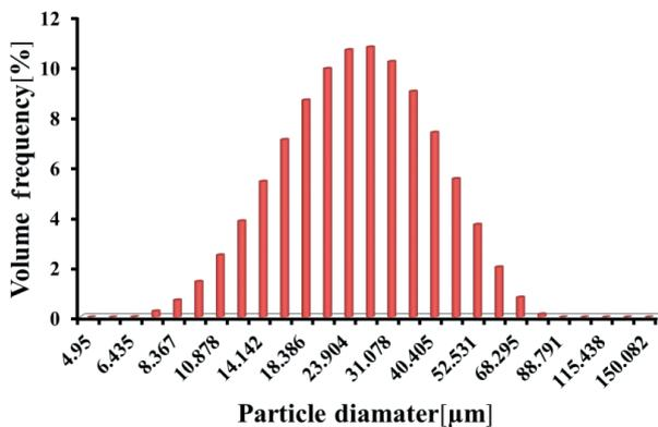
Figure 6 Diameter distribution of Titanium particles
