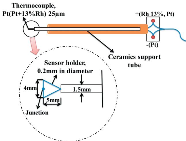
Figure 3 Structure of the thermocouple
