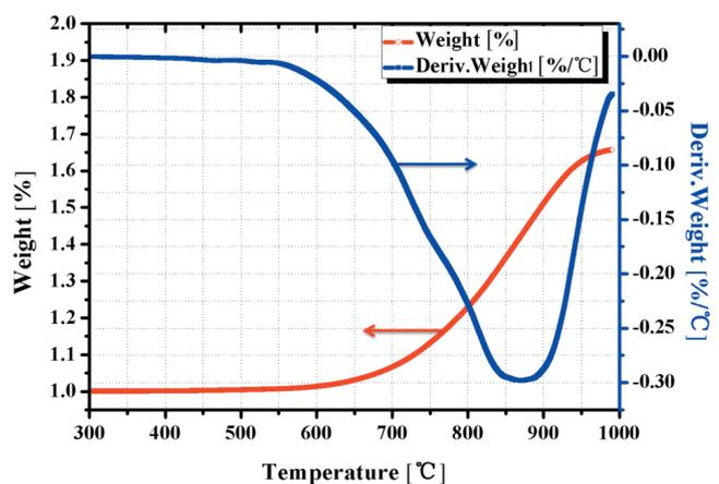
Figure 4 TGA profile of Titanium particles
