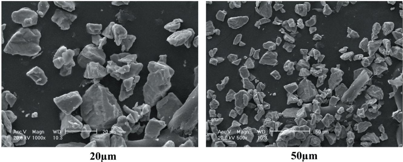
Figure 5 SEM photographs of Titanium particles
