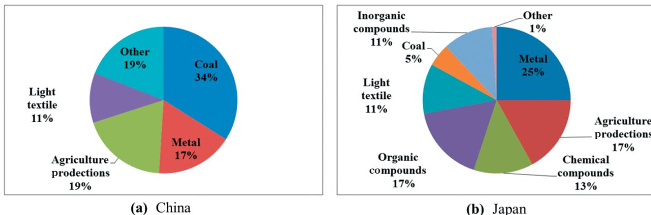
Figure 1 Industry distribution of dust explosions in China and Japan
