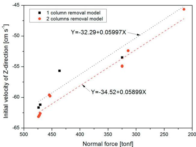
**Figure 14** The relationship between initial velocity and normal force applied on top of the removed columns.
