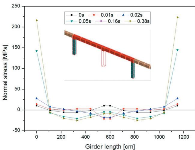
**Figure 9** Normal stress distribution along top bars in the girder of 1 internal column model.
