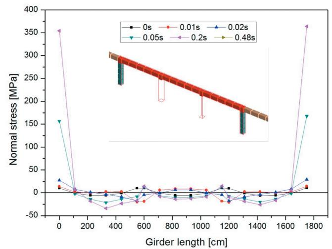
**Figure 11** Normal stress distribution along top bars in the girder of 2 internal column model.
