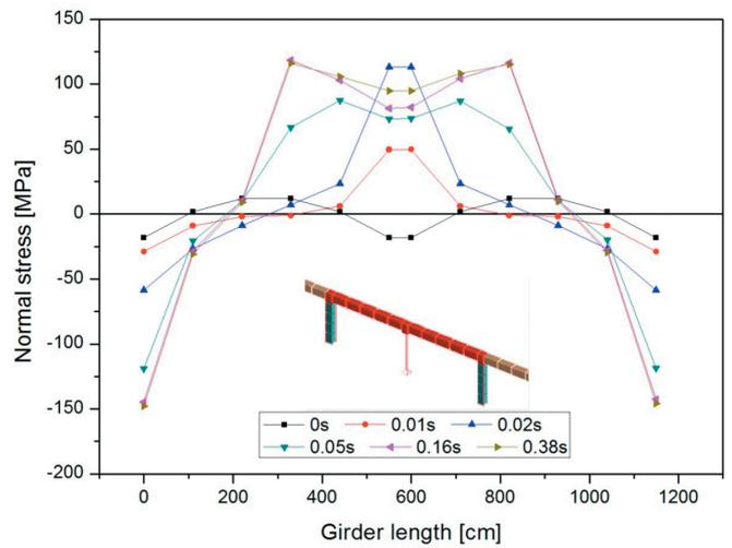
**Figure 10** Normal stress distribution along bottom bars in the girder of 1 internal column model.
