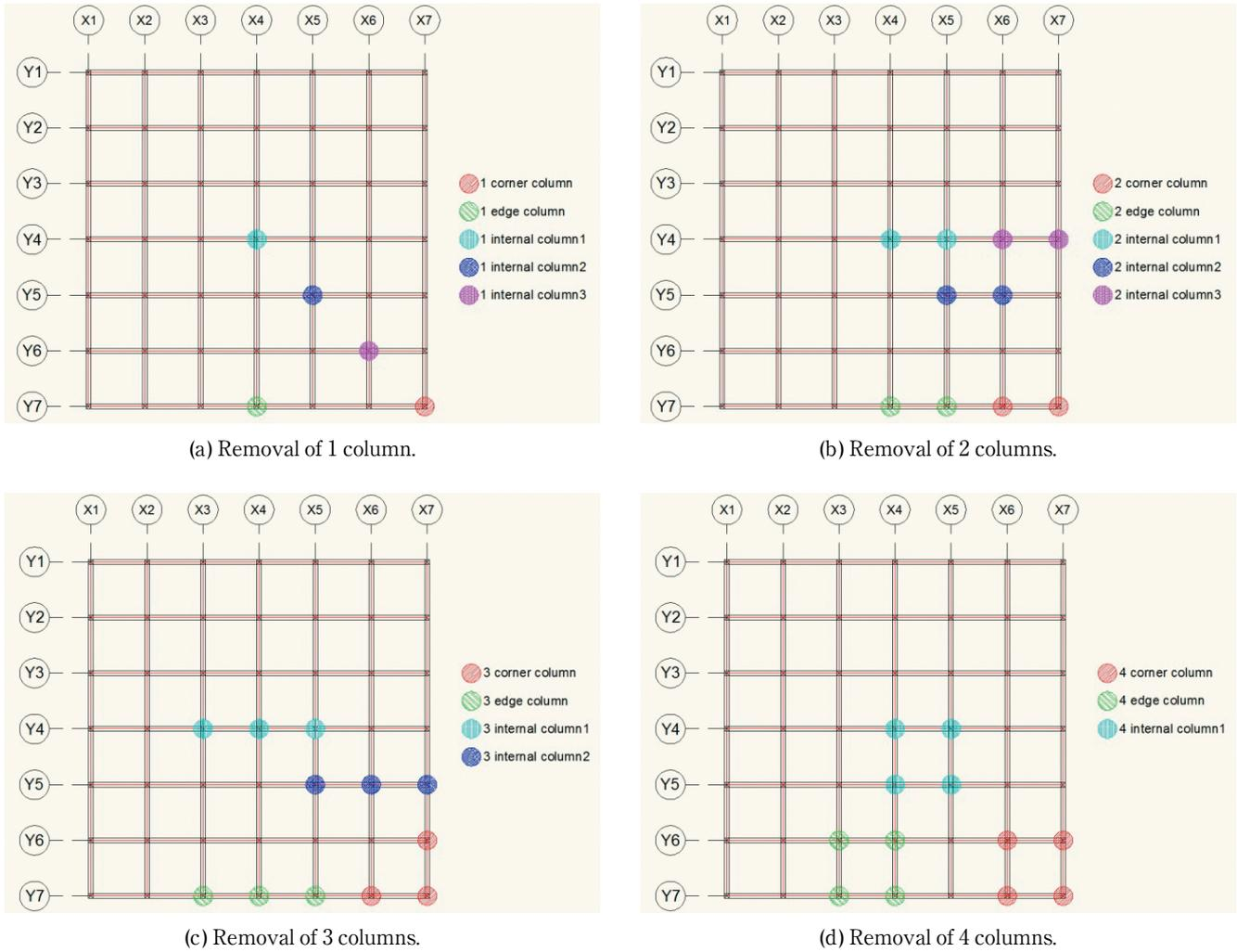
Figure 7 Position of columns to remove for each analysis model.
