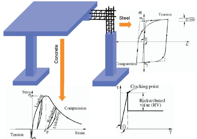
Figure 2 Constitutive models for concrete and reinforcing bar (Tagel-Din, 2009).
