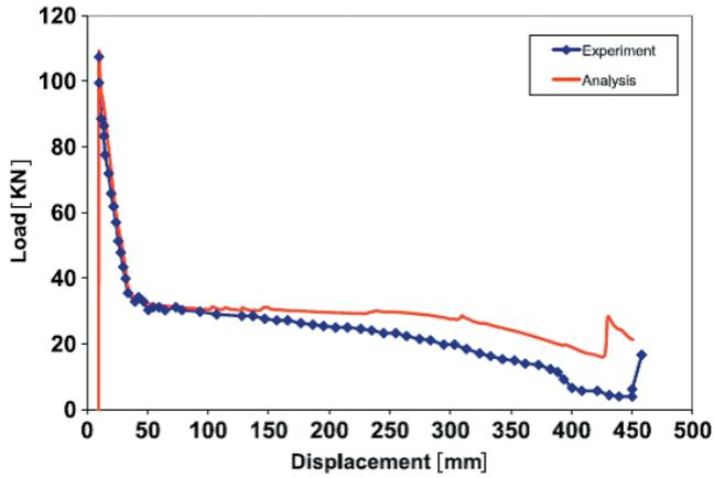
Figure 3 Middle column load vs. displacement of removed column predicted by AEM compared to the experimental results of Wei et al. (Salem et al., 2011).
