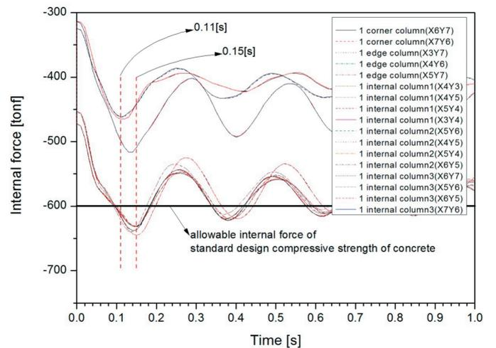
**Figure 15** The relationship between the vertical internal forces applied to the surrounding columns and time at 1 column removal models.
