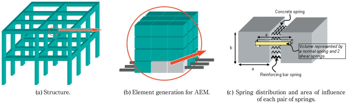
Figure 1 Modeling of structure to AEM (Tagel-Din, 2009).
