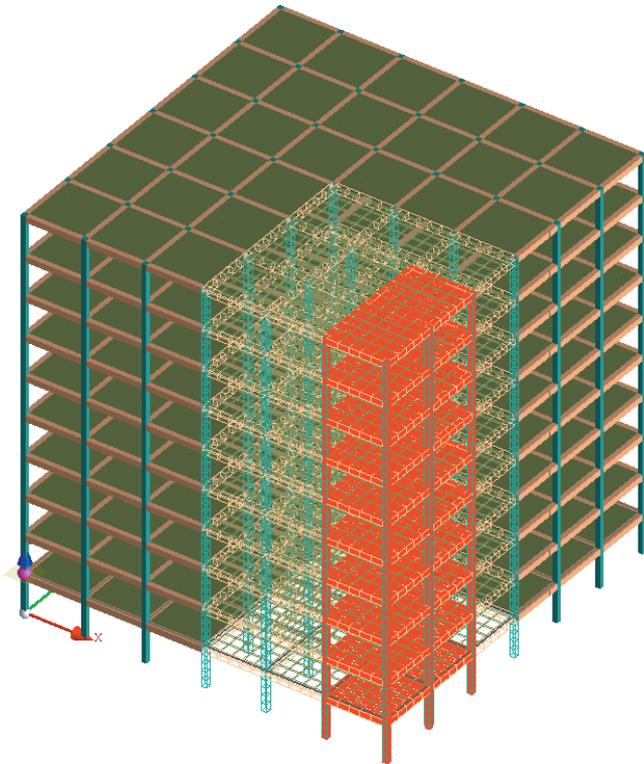
**Figure 6** AEM model for the concrete and reinforcing bars.
