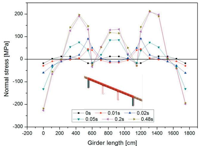
**Figure 12** Normal stress distribution along bottom bars in the girder of 2 internal column model.
