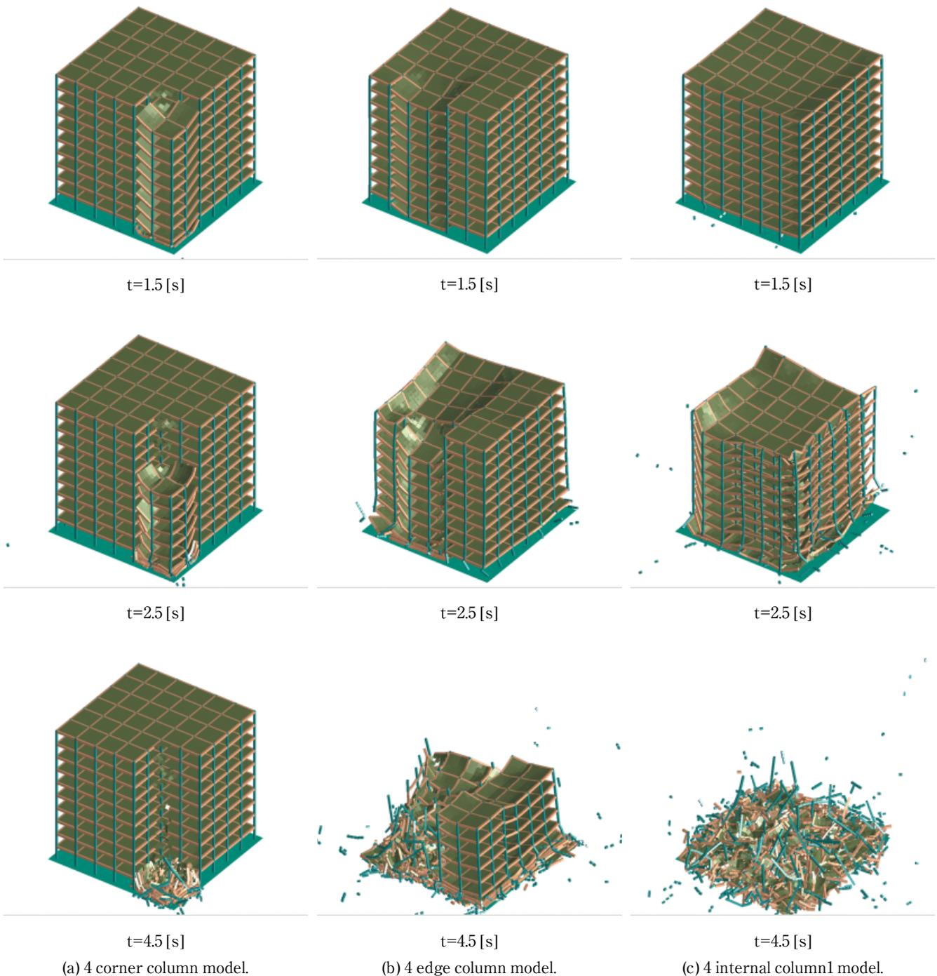
**Figure 13** Collapse behavior of 4 columns removal models according to analysis time.
