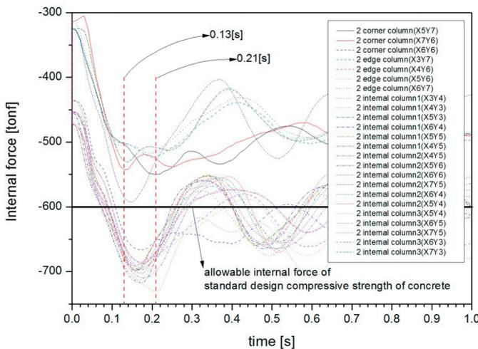
**Figure 16** The relationship between the vertical internal forces applied to the surrounding columns and time at 2 columns removal models.
