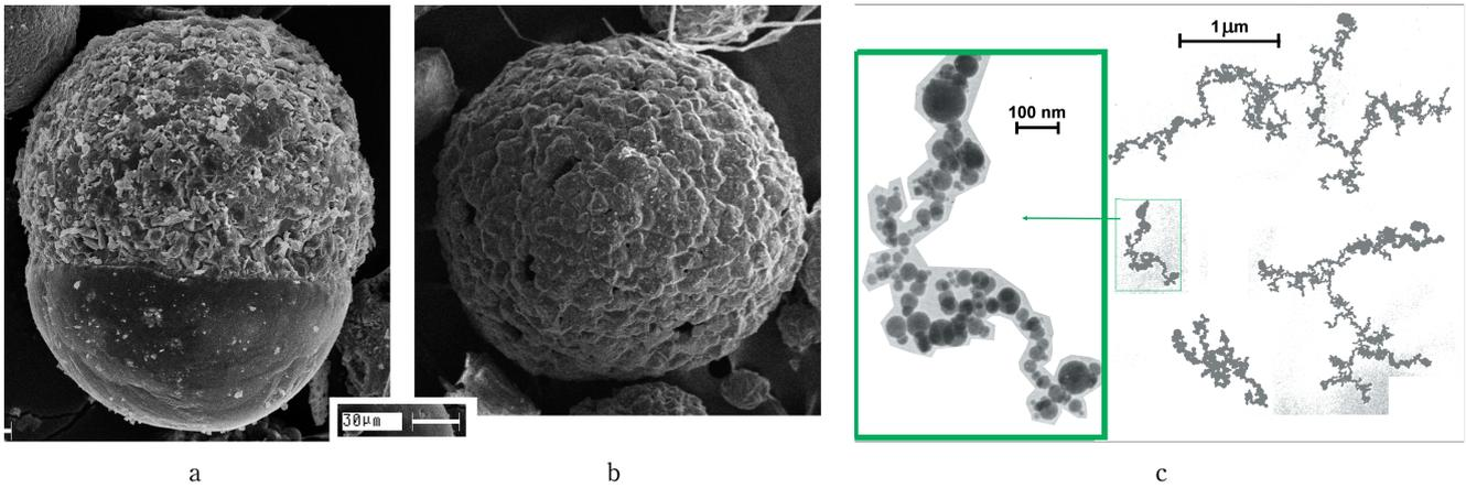
**Figure 3** Different size CCP particles: a) - acorn shaped agglomerate of 300 micron size quenched at the early stage of the combustion (unburned Al is on the bottom, oxide cup on the top); b) - same size agglomerate quenched at the final stage of the combustion, totally consisted of oxide; c) - micron-sized fractal aggregates composed of spherules - primary nano-sized oxide particles.
