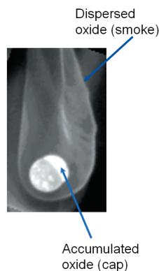
**Figure 1** Agglomeration and formation of condensed combustion products are characteristic features of aluminized propellants combustion.
