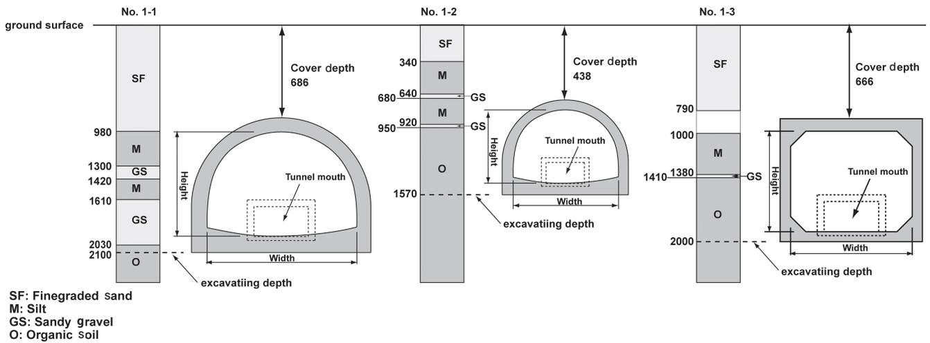
**Figure 1** Schematic drawings of the arch-shaped and box-shaped storage chambers with culvert structures (top). Installation conditions of the chamber and soil classification of surrounding ground (bottom, in cm).
