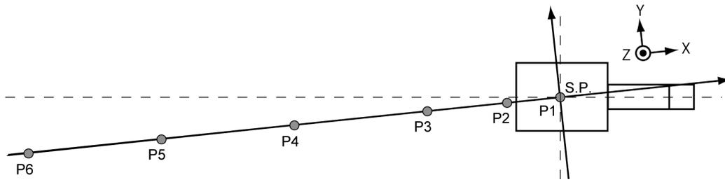
**Figure 3** Layout of accelerator sensors and reference axes for vibration measurement.
