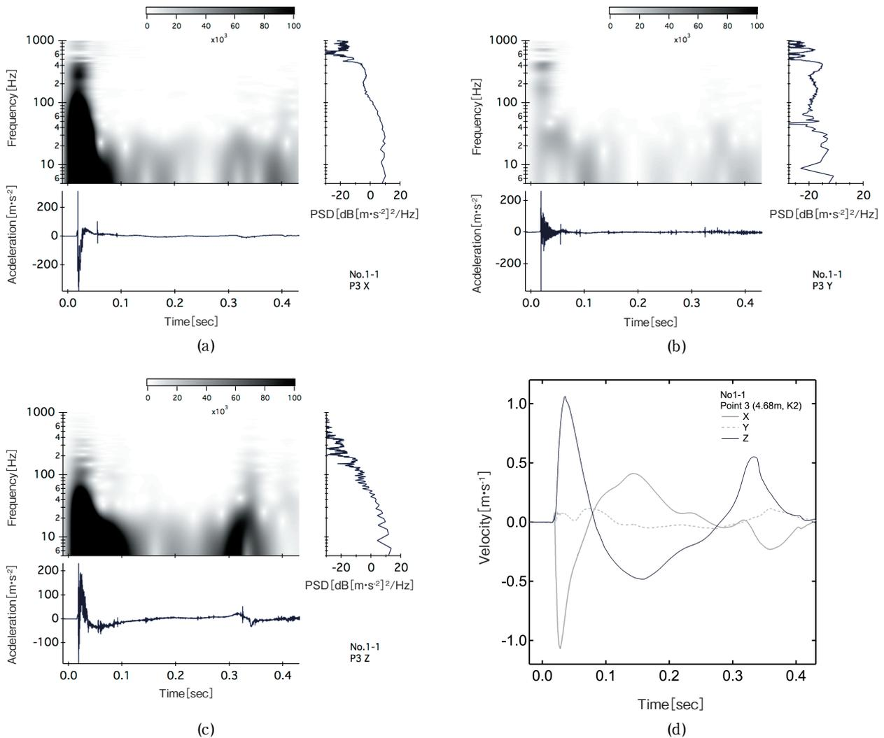
**Figure 5** (a)-(c) Measured acceleration signals and analyzed sonogram and power spectrum density (PSD) for x, y, and z directions (a: X, b: Y, c: Z). (d). Integrated vibration velocity (V). (test No. 1-1, point P3, distance 4.68 m, K2).
