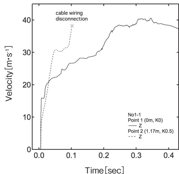
**Figure 6** Integrated vibration velocity profile (test No. 1-1, points P1 and P2).
