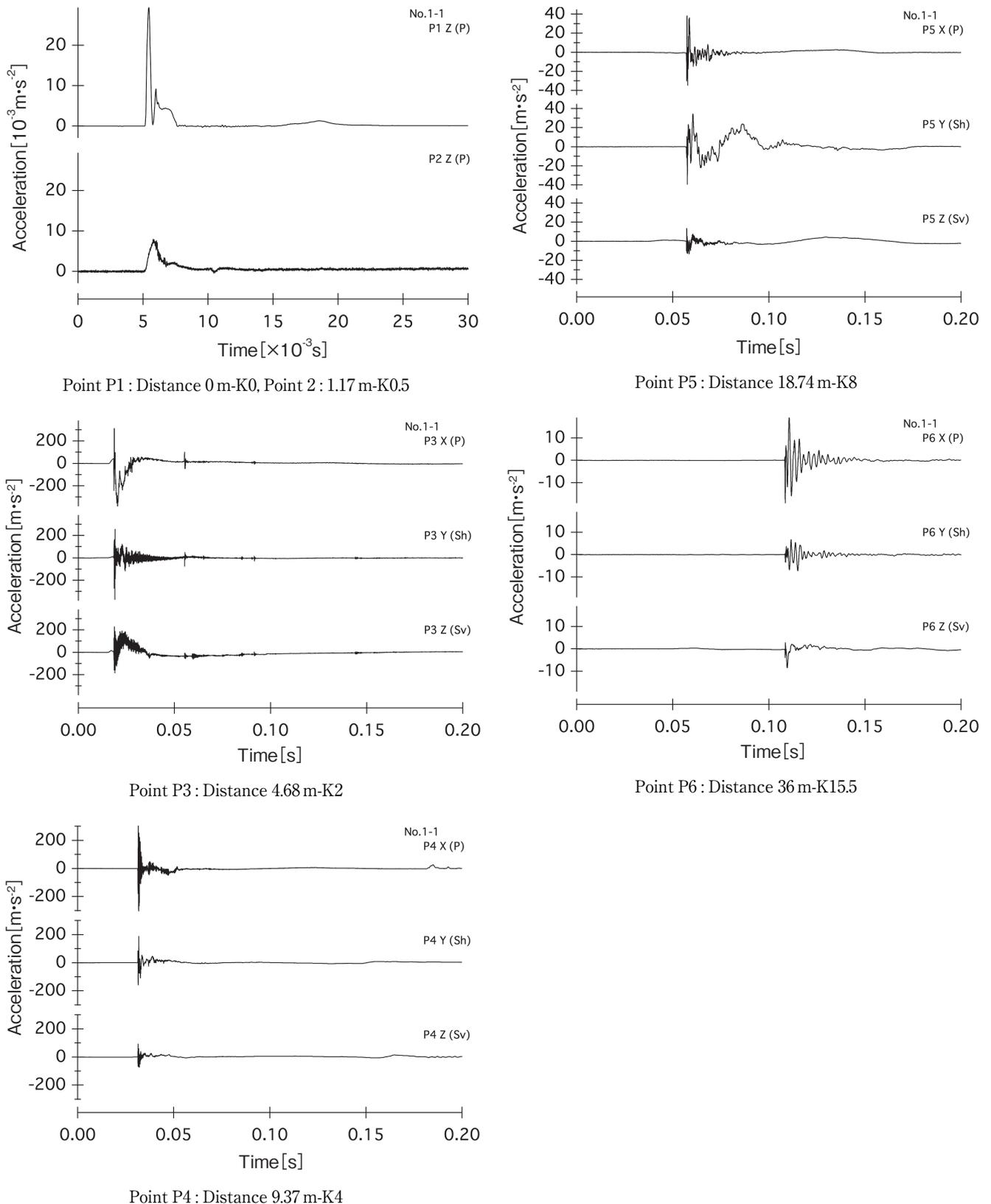
**Figure 4** Measured acceleration signals in x, y, and z directions for test No. 1-1.
