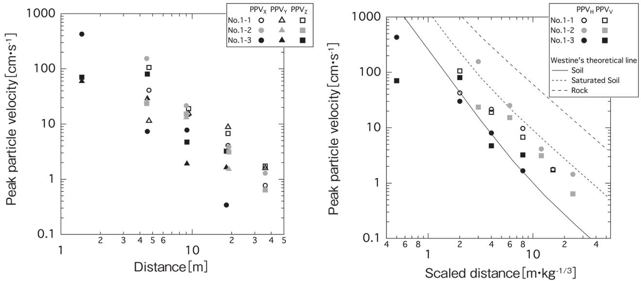
**Figure 7** Peak particle velocity (PPV) for x, y, and z directions plotted against distance (left) and for horizontal and vertical directions plotted against scaled distance (right).
