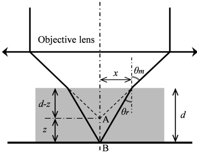
Figure 1 Schematic of the Duc de Chaulnes method.
