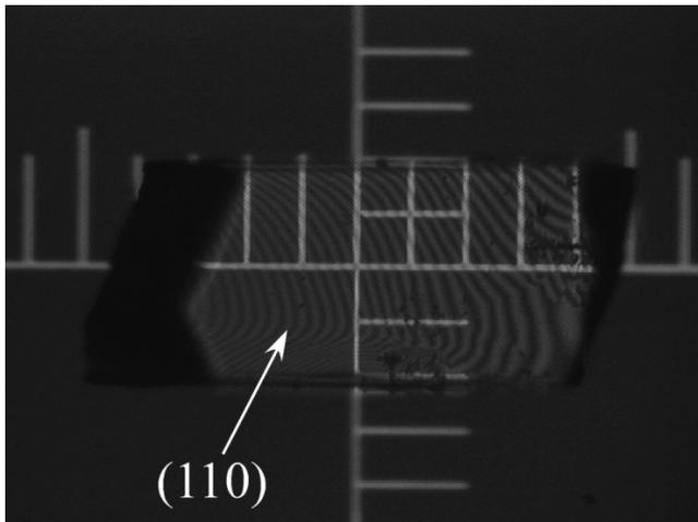
**Figure 3** Micrograph of a PETN single crystal (110) illuminated at 532 nm using a 10× objective lens. The smallest increment on the scale is 100 μm.
