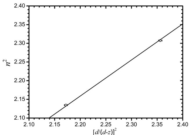
Figure 2 Relationship between  $n^2$  and  $[d/(d-z)]^2$  used to calibrate the microscope at a wavelength of 532 nm. Measured data points for the  $\text{SiO}_2$  and BK7 glass samples are indicated. The error bars are due to the uncertainty in the displacement of the image.
