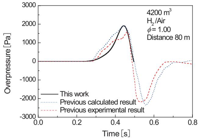
**Figure 2** Comparison of blast wave histories between the previous experimental results and the calculated result in this study for a large-scale experiment.
