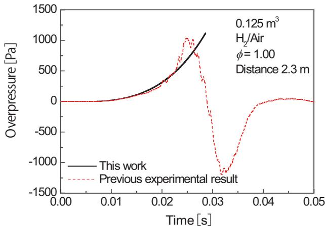
**Figure 1** Comparison of blast wave histories between the previous experimental results and the calculated result in this study for a small-scale experiment.
