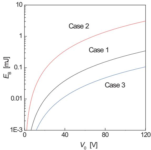
**Figure 4** Dependence of energy consumed in bridgewire ( $E_B$ ) on battery voltage ( $V_0$ ).
