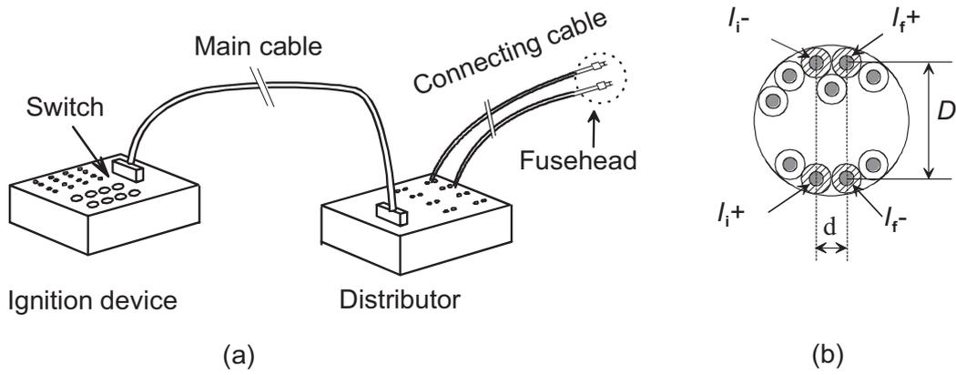
**Figure 1** Typical electric ignition system for launching fireworks (a) and cross-sectional view of a multi-conductor cable used in the system (b).
