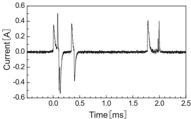
**Figure 5** Time profile of induced current caused by chatter in mechanical switch.
