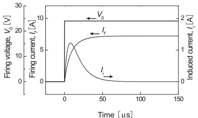
**Figure 3** Time profiles of firing current,  $I_f$ , and induced current,  $I_i$ , when a voltage,  $V_0$ , is applied instantaneously. Values of the parameters used in the calculation are as follows:  $V_0 = 24.0$  V,  $R_1 = 2.72$   $\Omega$ ,  $L_1 = 31.5$   $\mu$ H,  $M = 11.7$   $\mu$ H,  $R_2 = 2.97$   $\Omega$  and  $L_2 = 24.7$   $\mu$ H.
