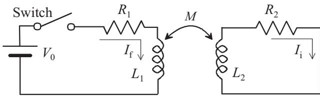
**Figure 2** Electrical circuit representing electromagnetic induction effect in ignition system.
