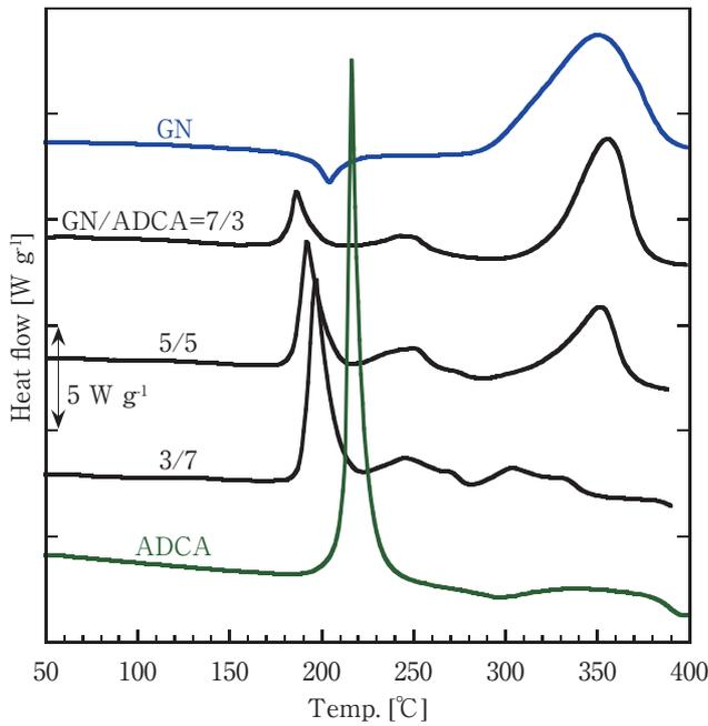
**Figure 3** Sealed cell DSC curves of GN, ADCA and ADCA/GN compositions.
