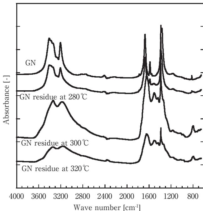
**Figure 7** FT-IR spectra of GN and its decomposition residue at 280°C, 300°C and 320°C.
