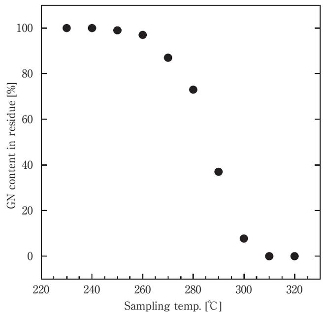
**Figure 6** Ratio of GN remained in GN decomposition residue at sampling temperatures.
