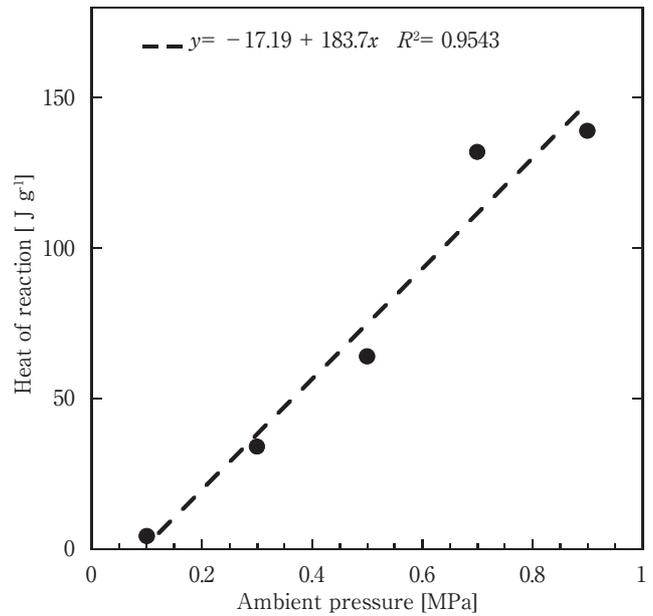
**Figure 5** Plots of heat of reaction vs. ambient pressure of GN.
