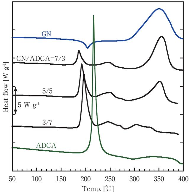
**Figure 3** Sealed cell DSC curves of GN, ADCA and ADCA/GN compositions.
