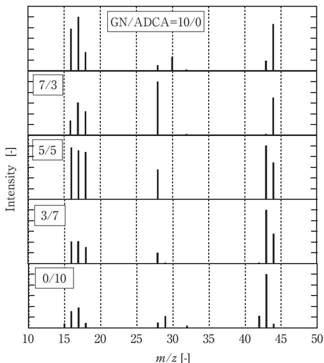
**Figure 10** Mass spectra of gases evolved from GN, ADCA and GN/ADCA compositions at above 260 °C.
