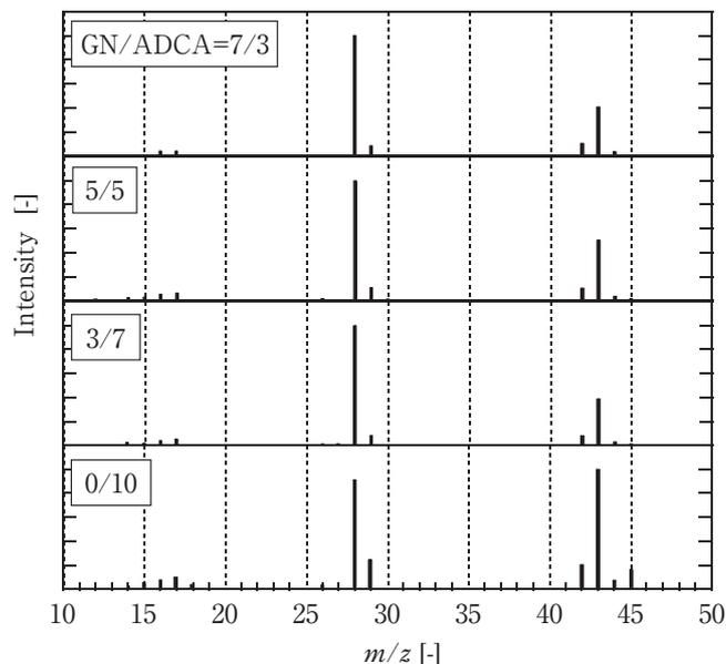
**Figure 9** Mass spectra of gases evolved from ADCA and GN/ADCA compositions at around 200°C.
