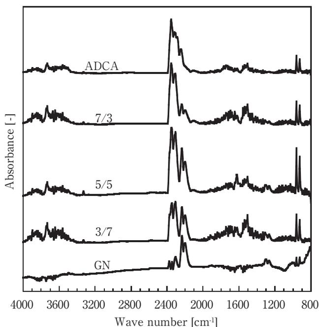
**Figure 8** FT-IR spectra of gases evolved from GN, ADCA and GN/ADCA compositions.
