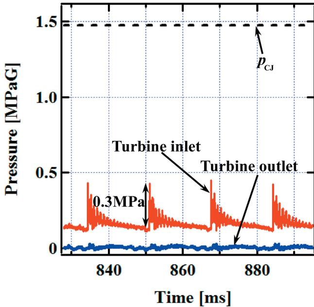
Figure 2 Pressure histories at the turbine inlet and outlet (operation frequency : 60 Hz).
