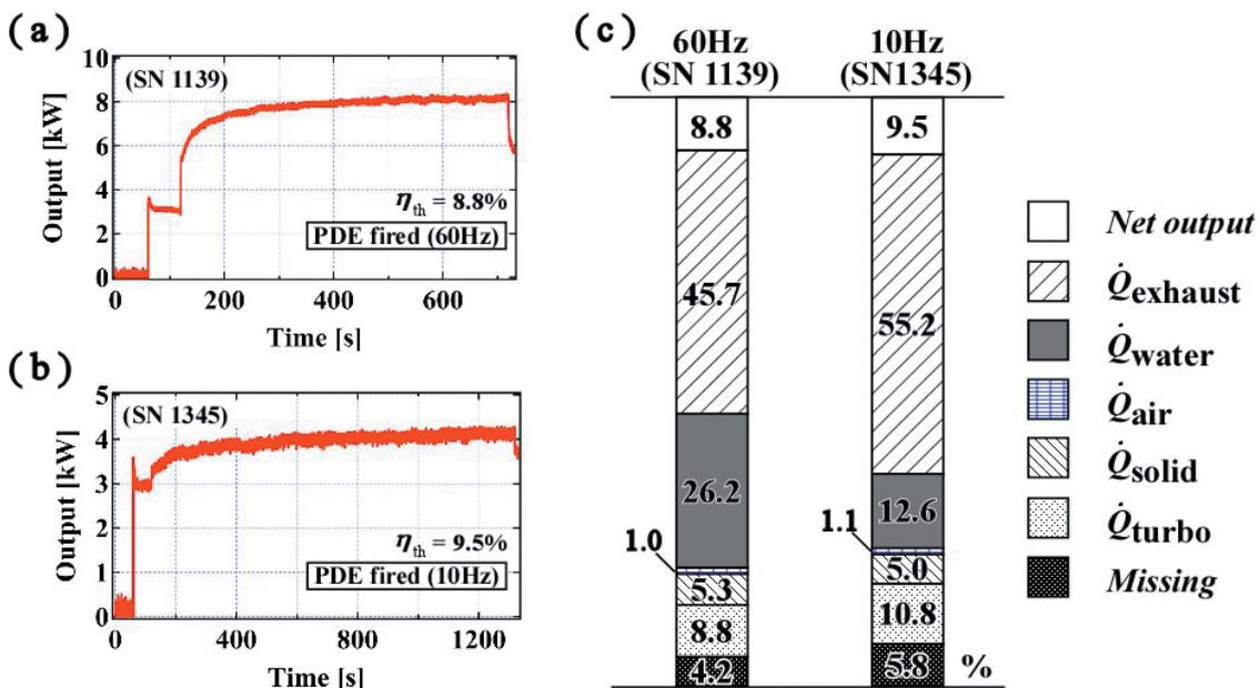
Figure 4 Experimental results on the energy balance. (a) Time history of the output for the 60-Hz case. (b) Time history of the output for the 10-Hz case. (c) Energy balance.
