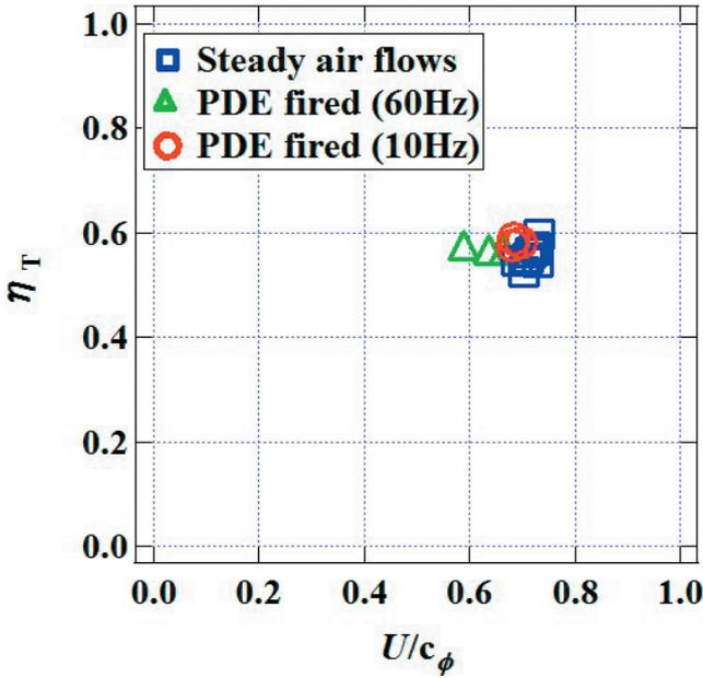
Figure 3 Isentropic efficiency of the turbocharger.
