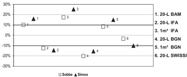
**Fig. 5** Differences of  $K_{St}$ -values for tests with Maize starch in 20-L-sphere and 1-m<sup>3</sup>-vessel.
