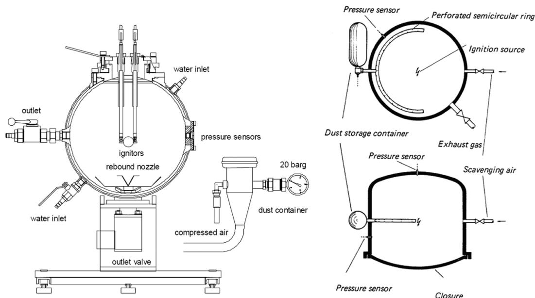
**Fig. 1** Schematic of standard 20-L-sphere (left side) and front view (upper right side) and top view (lower right side) of 1-m<sup>3</sup>-vessel (VDI 2263-1<sup>5</sup>).
