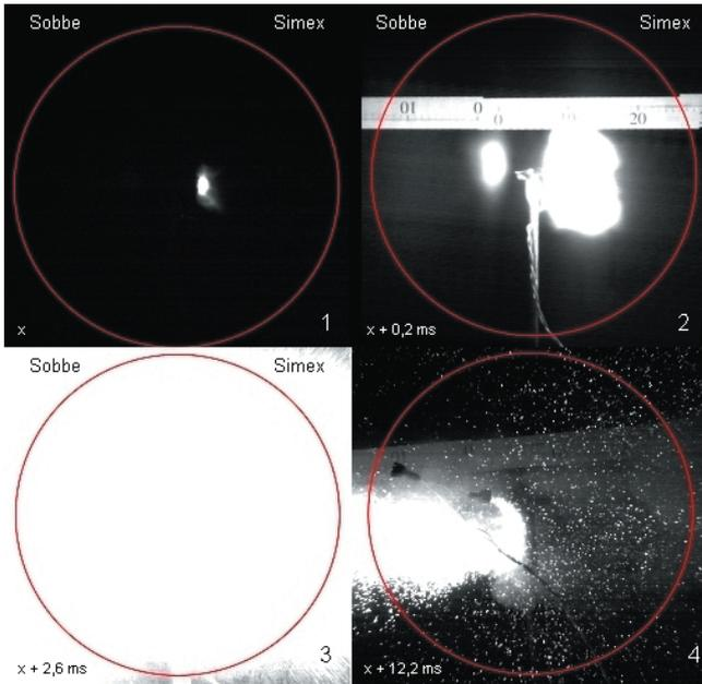
**Fig. 3** Flame propagation of both igniters, photos filmed with high speed camera at time  $x$ ,  $x + 0.2$  ms,  $x + 2.6$  ms and  $x + 12.2$  ms.
