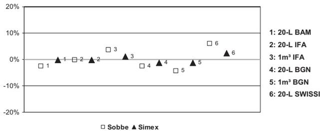
**Fig. 4** Differences of  $P_{max}$  for tests with Niacin in 20-L-sphere and 1-m<sup>3</sup>-vessel.
