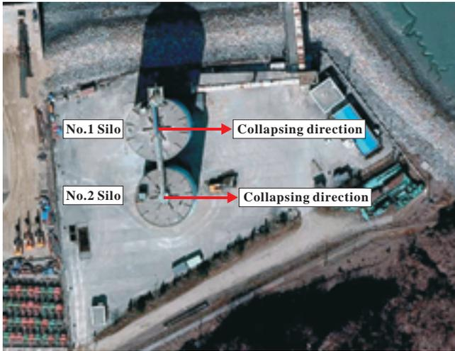
Fig. 4 Expected collapsing direction of the target structure for explosive demolition.
