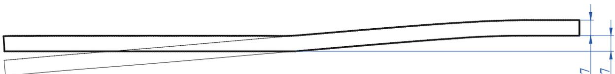
Fig. 7 Transient deflection profiles of a free (thin line) and a colliding (thick line) flyer plate obtained from numerical analysis.
