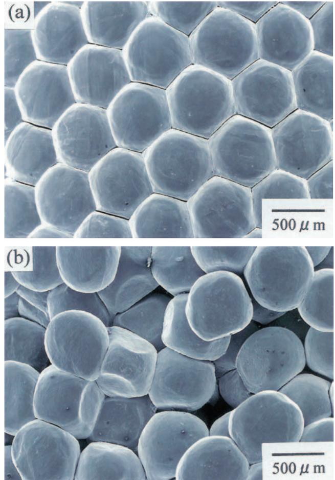
Fig. 4 SEM micrographs of Ti porous-surfaced implants, (a) T 6 and (b) T 6 M73.
