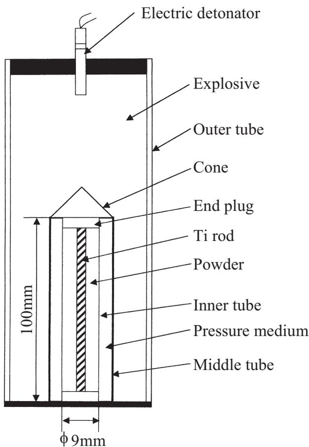
Fig. 2 Assembly for cylindrical explosive compaction.
