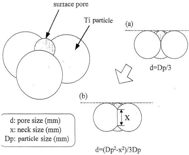
Fig. 3 Concept of surface pore size in this study.
