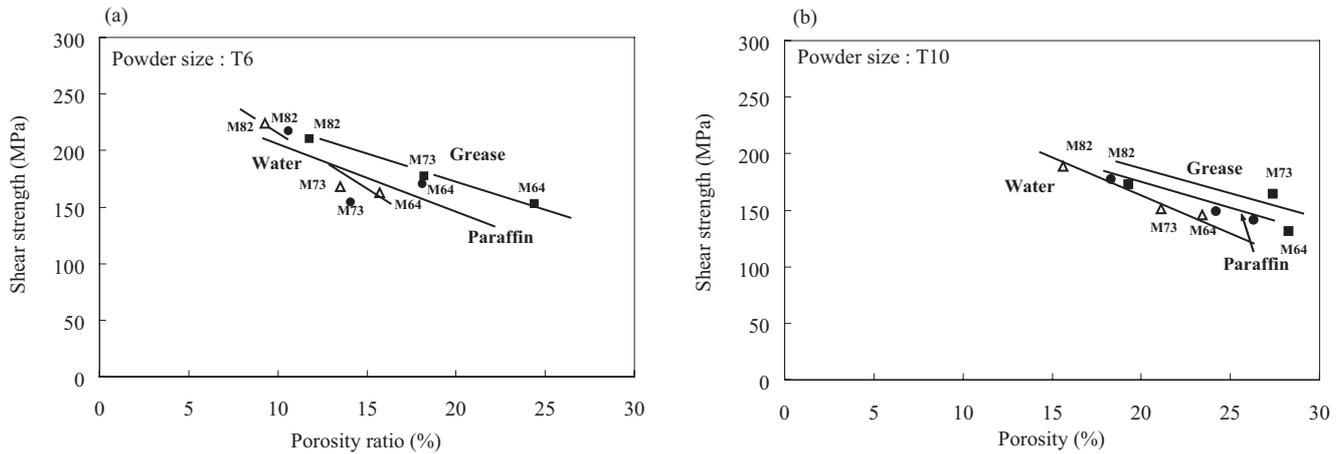
Fig. 6 The relationship between shear strength and porosity ratio using various transmitting media. (a) T6 particle and (b) T10 particle.
