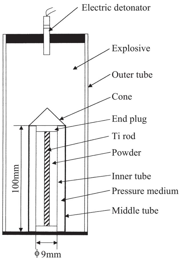
Fig. 2 Assembly for cylindrical explosive compaction.
