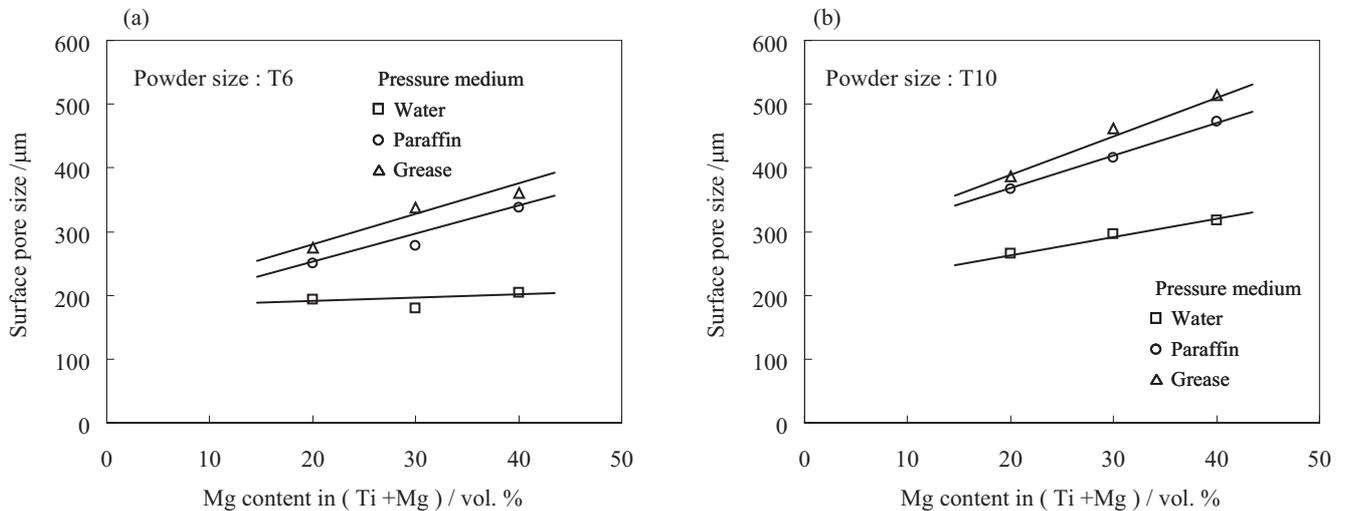
Fig. 5 The relationship between surface pore size and Mg content in (Ti+Mg) content using various transmitting pressure media, (a) T 6 particle and (b) T10 particle.
