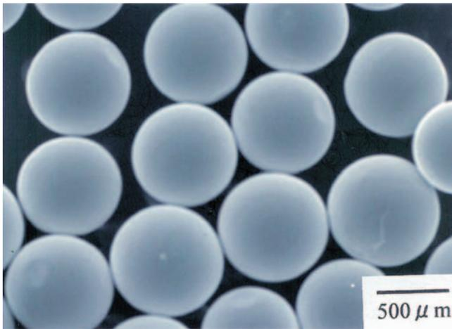
Fig. 1 SEM micrograph of titanium particles with diameter of T 6 (610µm).
