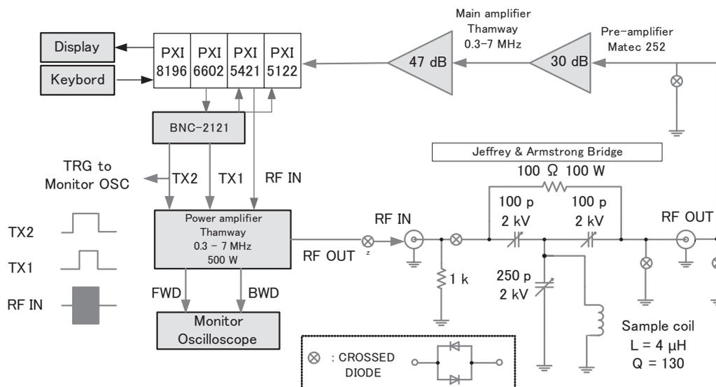
Fig. 1 Block diagram of a PC-controlled pulse Fourier-transform NQR spectrometer
