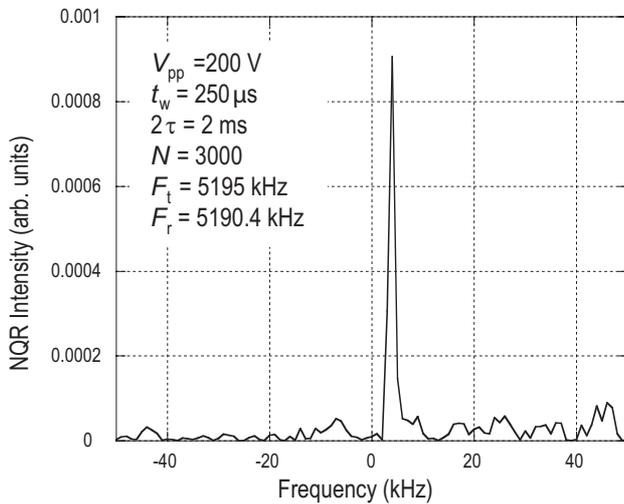
**Fig. 5** The one of  $\nu_+$  lines (5192 kHz at RT) obtained from 300 g of RDX located 3.5 cm above the gradiometer coil by the FFT method under unshielded circumstance. The abscissa is the offset from the reference frequency.
