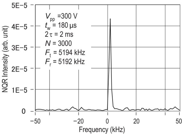
**Fig. 6** The one of  $\nu_+$  lines (5192 kHz at RT) obtained by the FFT method from 300 g of RDX in a large volumetric solenoid. The abscissa is the offset from the reference frequency.
