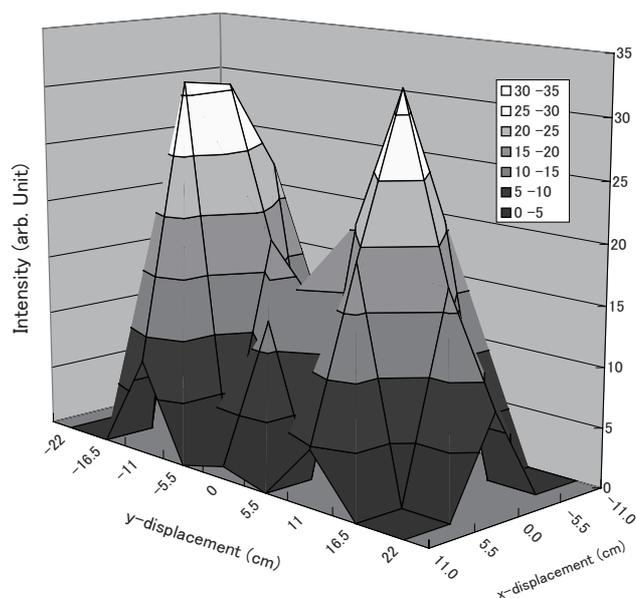
Fig. 3 Positional dependence of the NQR signal amplitude from 500 g of NaNO<sub>2</sub> on the surface of the gradiometer coil. The measurements conditions by SORC pulse sequence were  $V_{pp} = 200$  V,  $t_w = 100$   $\mu$ s,  $2\tau = 2$  ms,  $N = 40000$ .
