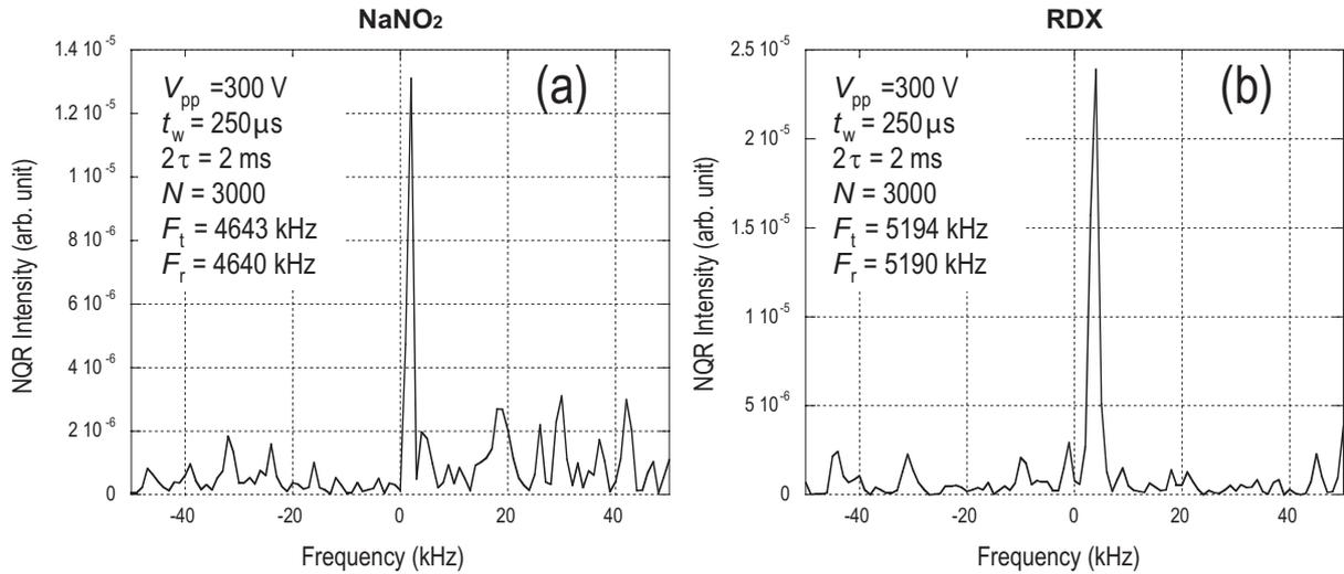
**Fig. 4** (a) The signal  $\nu_+$  (4640 kHz at RT) obtained from 500 g of NaNO<sub>2</sub> located 15.5 cm above the nonlinear spiral coil. (b) The one of  $\nu_+$  lines (5192 kHz at RT) obtained from 300 g of RDX located 8.5 cm above the nonlinear spiral coil. In the insert legend,  $F_t$  and  $F_r$  denote the transmitter and reference frequencies, respectively. The abscissa is the offset from the reference frequency.
