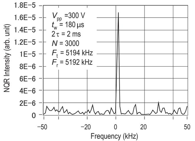
**Fig. 7** The one of  $\nu_+$  lines (5192 kHz at RT) from 300 g of RDX in a baggage which contains a stainless steel tray under the RDX and metallic tools. The abscissa is the offset from the reference frequency.
