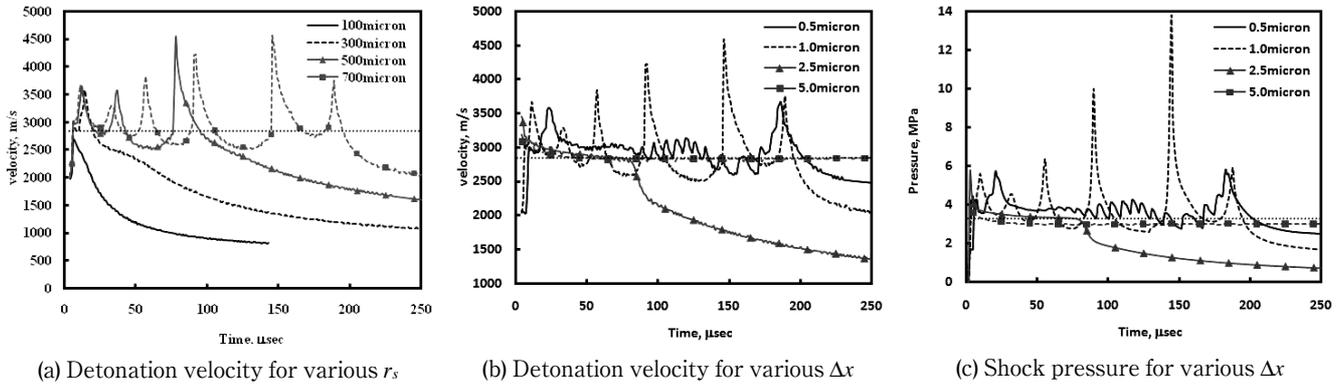
Fig. 1 Time history of detonation velocity and shock pressure.  $\Delta x=1.0\mu\text{m}$  in Fig.1(a) and  $r_s=700\mu\text{m}$  in Fig.1(b) and (c).
