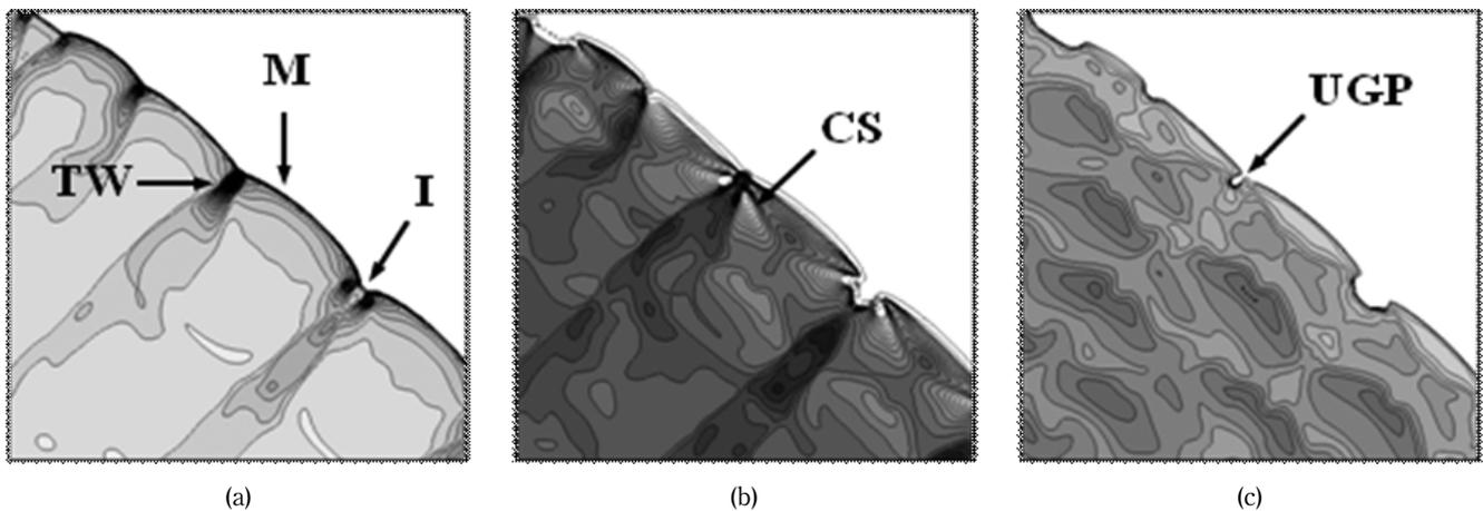
Fig. 4 Contours near the detonation front for  $r_s=700\mu\text{m}$  and  $\Delta x=5.0\mu\text{m}$ . (a) pressure, (b) temperature and (c)  $\text{H}_2$  mass fraction distribution. The gray regions in Fig.4(a) and (b) and the white regions in Fig.4(c) denote high values. I: incident shock, M: Mach stem, TW: transverse wave, CS: contact surface, and UGP: unburned gas pocket.
