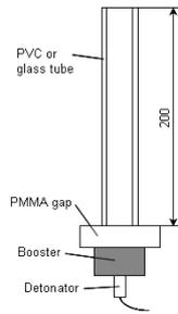
Figure 1 Assembly for optical method experiments.
