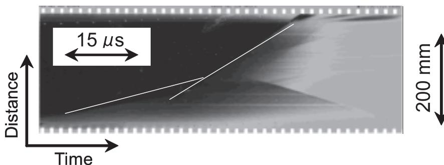
Figure 3 An example of a streak photograph obtained by the optical method (PVC tube, 15 mm gap).
