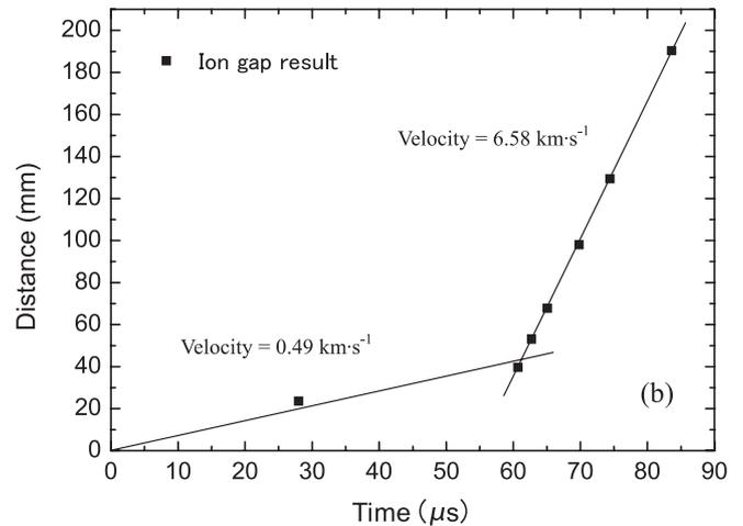
**Figure 5** Relation of time and distance obtained by the electrical method (a) :PVC tube, 15 mm gap, (b) :PVC tube, 20 mm gap.
