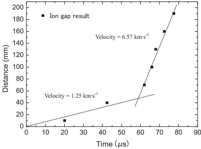
**Figure 4** Relation of time and distance obtained by the electrical method (glass tube, 15 mm gap).
