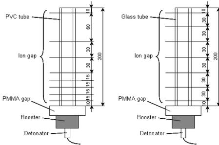
Figure 2 Assembly for electrical method experiments.
