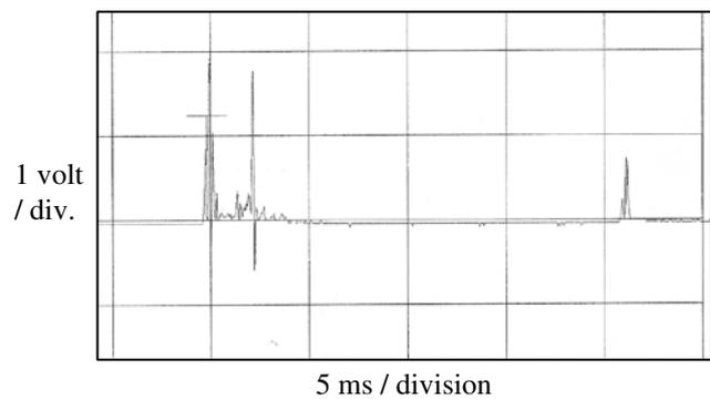
**Fig. 2** Shock and gas waves of Cu- instantaneous detonator.**Table 2** Shock and gas energy of detonating fuse.
