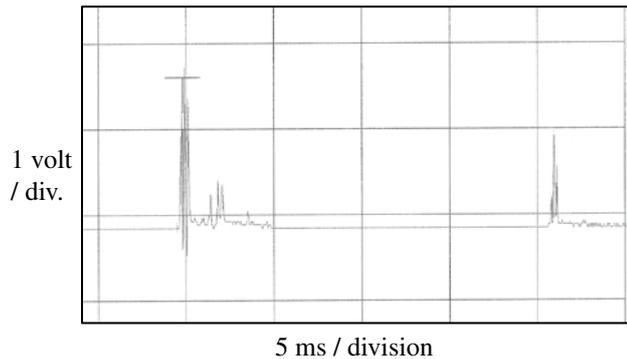
**Fig. 1** Shock and gas waves of Al- instantaneous detonator.
