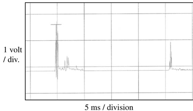
**Fig. 1** Shock and gas waves of Al- instantaneous detonator.
