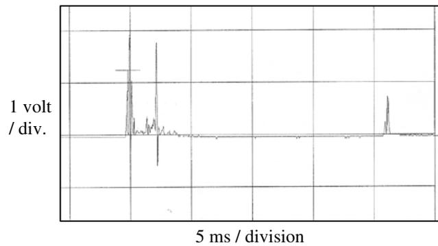
**Fig. 2** Shock and gas waves of Cu- instantaneous detonator.**Table 2** Shock and gas energy of detonating fuse.
