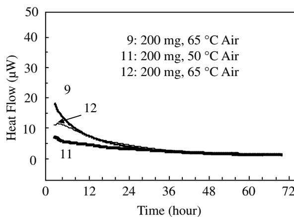
Fig. 5 Heat flow of magnesium powder in two temperatures measured with 4 ml vessels.
