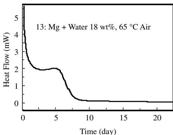
Fig. 6 Heat flow of magnesium powder added with water measured with 20 ml vessels.
