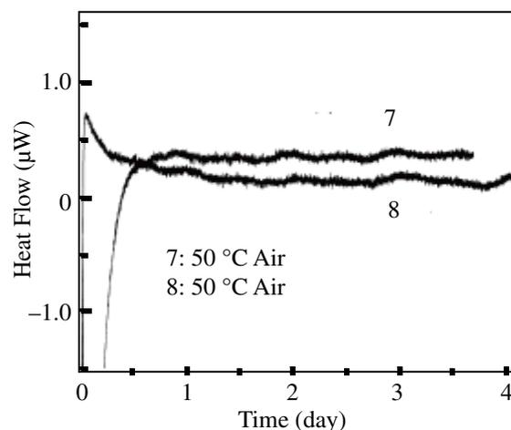
Fig. 3 Heat flow of magnesium turnings measured with 20 ml vessels.
