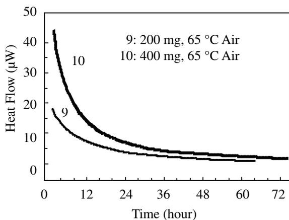
Fig. 4 Heat flow of magnesium powder in two amount of sample measured with 4 ml vessels.
