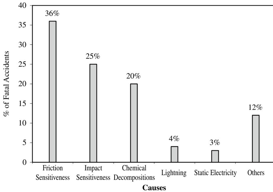
Fig. 3 Accidents due to causes in the manufacturing of fireworks during 1994-2006.
