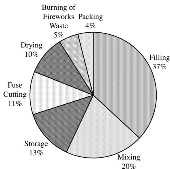
Fig. 2 Accidents in fireworks manufacturing, during 1994-2006.
