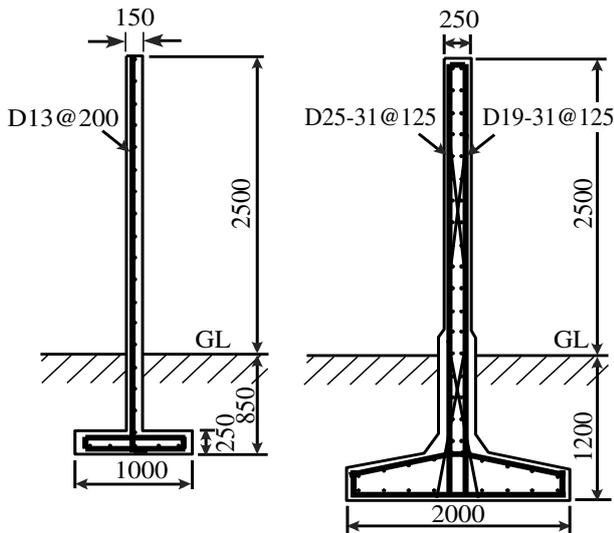
Fig. 1 Two kinds of concrete walls. (a) conventional concrete wall for experiment #2, and (b) high-strength concrete wall for experiment #3.
