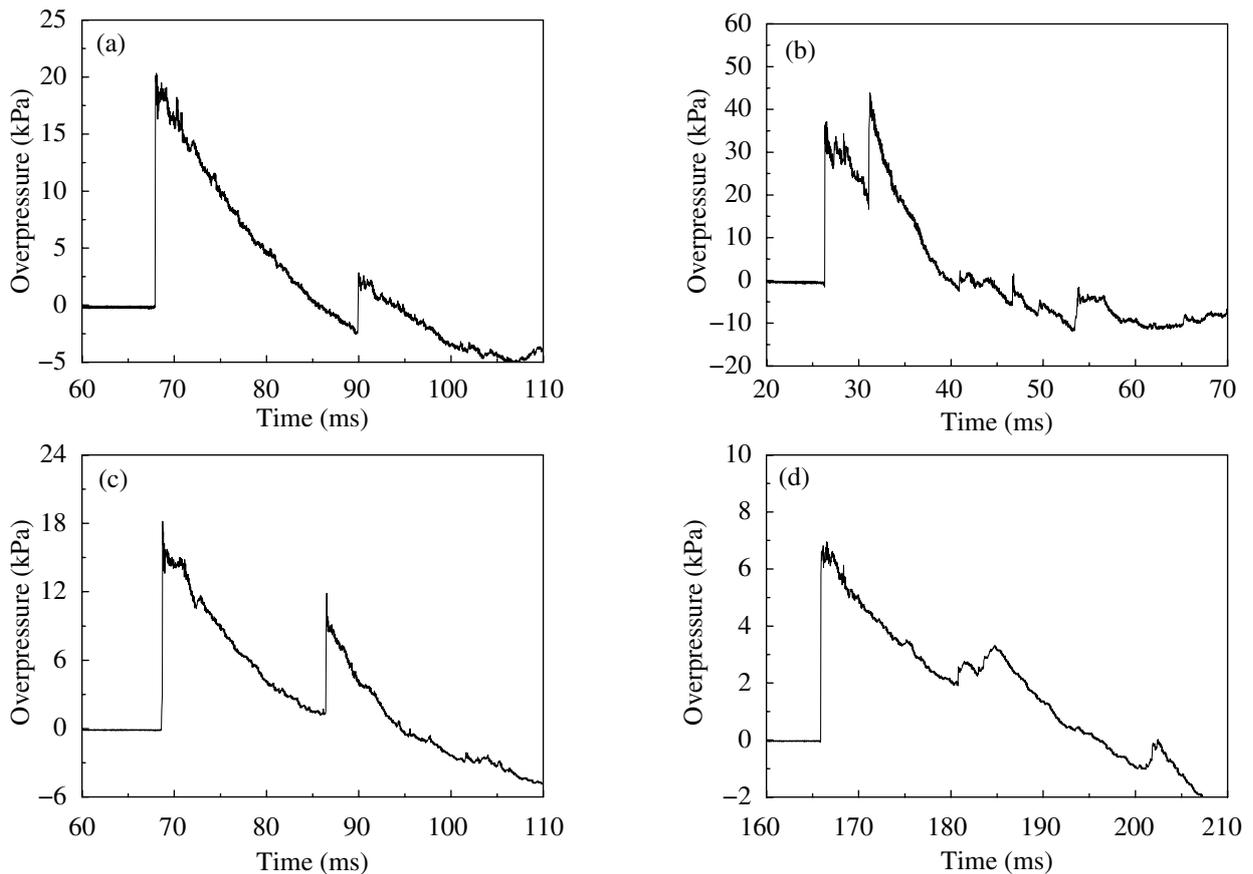
(a) Typical wave profile of the surface burst of experiment # 1 at  $\theta = 90^\circ$  and  $K = 8$ .
