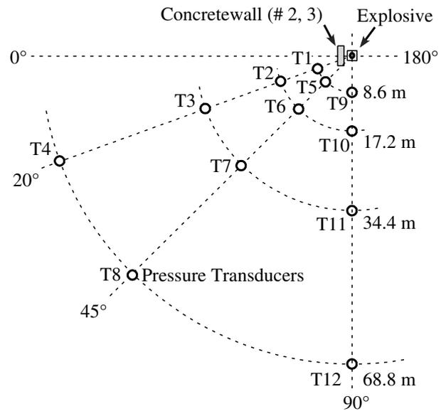
Fig. 2 Setup of blast pressure measurement on the experiment field. T1-T12 correspond to the transducer number.
