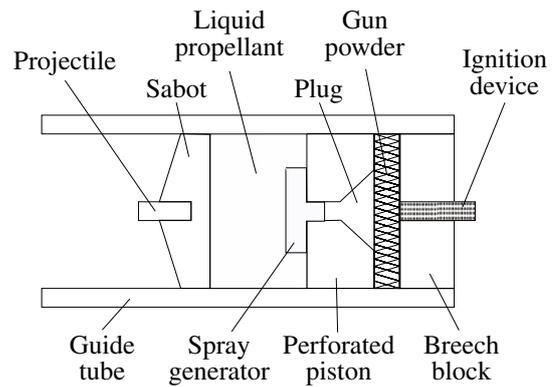
Fig. 2 Travelling liquid charge accelerator with ignition device.
