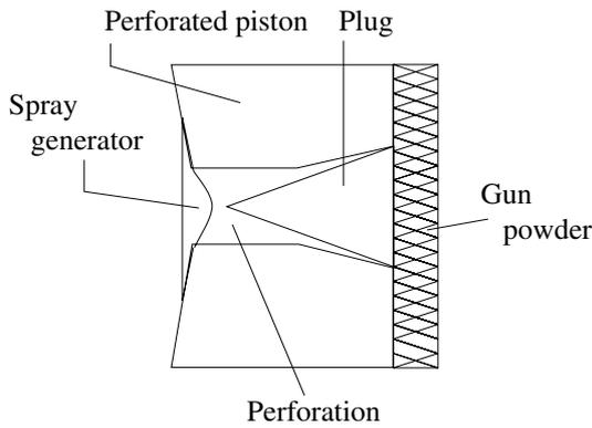
Fig. 1 Perforated piston with plug and a spray generator.
