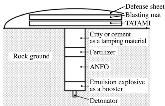
Fig. 1 The loading aspect of ANFO and fertilizer.
