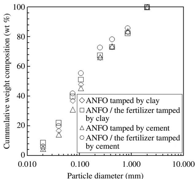
Fig. 4 The weight cumulative curves of less than 2 mm size particles at the bottom of the crater.
