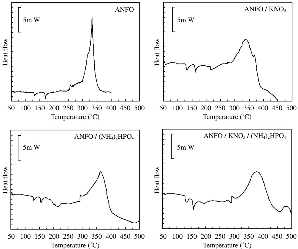
Fig. 2 The thermal behaviors of ANFO and ANFO with the fertilizer.
