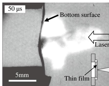
Fig. 11 High speed photographic records of the combustion process of multi-layered LS / CTA reactive film. Mass ratio LS / CTA is 8 : 2 with 200  $\mu\text{m}$  in thickness. Laser fluence is 30  $\text{J cm}^{-2}$ .
