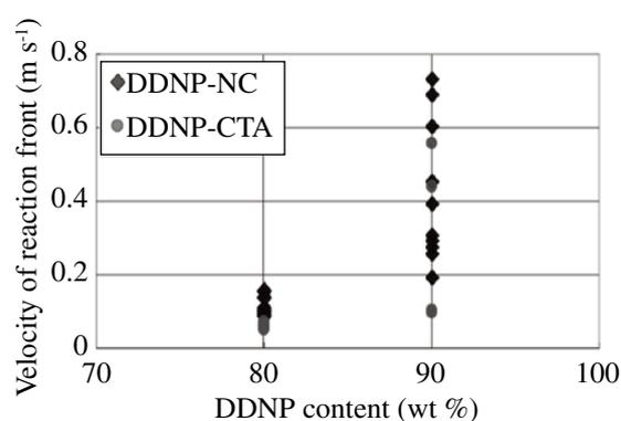
Fig. 12 Reaction front velocity of DDNP / CTA and DDNP / NC reactive thin films. Laser fluence for DDNP / CTA films is 30  $\text{J cm}^{-2}$ , while that for DDNP / NC films is 15  $\text{J cm}^{-2}$ , respectively.
