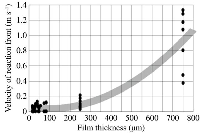
**Fig. 8** Reaction front velocity of DDNP / CTA reactive thin film as a function of film thickness. Mass ratio DDNP / CTA is 8 : 2. Laser fluence for all the data is 29-30  $\text{J cm}^{-2}$ .
