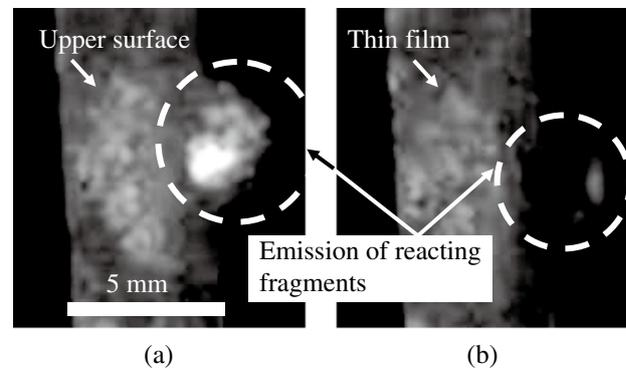
**Fig. 6** High speed video camera record of monolayer DDNP / CTA reactive thin film combustion process. Film specifications are as follows: DDNP / CTA = 8 / 2, and have  $32 \mu\text{m}$  in thickness prepared by PAD method. Pulse laser fluence is  $29 \text{ J cm}^{-2}$ . Delay time is (a)  $50 \mu\text{s}$  and (b)  $174 \mu\text{s}$  with gate time of  $2 \mu\text{s}$ .
