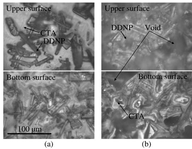
Fig. 2 Microscope pictures of upper and bottom surface of DDNP / CTA reactive thin film prepared by BC method. Mass ratio of DDNP / CTA is 8 : 2. (a) Monolayer film with 21  $\mu\text{m}$  thickness, and (b) monolayer film with 84  $\mu\text{m}$  thickness, respectively.
