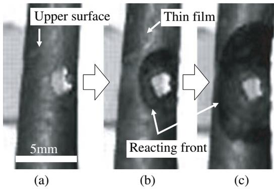
**Fig. 7** High speed video camera record of monolayer DDNP / CTA reactive thin film combustion process. Film specifications are as follows: DDNP / CTA = 8 / 2, and have 32  $\mu\text{m}$  in thickness prepared by PAD method. Pulse laser fluence is 29  $\text{J cm}^{-2}$ . Delay time is (a) 1ms and (b) 21 ms, 35 ms with gate time of 2  $\mu\text{s}$ .
