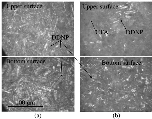
Fig. 1 Microscope pictures of upper and bottom surface of DDNP / CTA reactive thin film prepared by PAD method. Mass ratio of DDNP / CTA is 8 : 2. (a) Monolayer film with 19  $\mu\text{m}$  thickness, and (b) multi-layered film with 370  $\mu\text{m}$  thickness, respectively.
