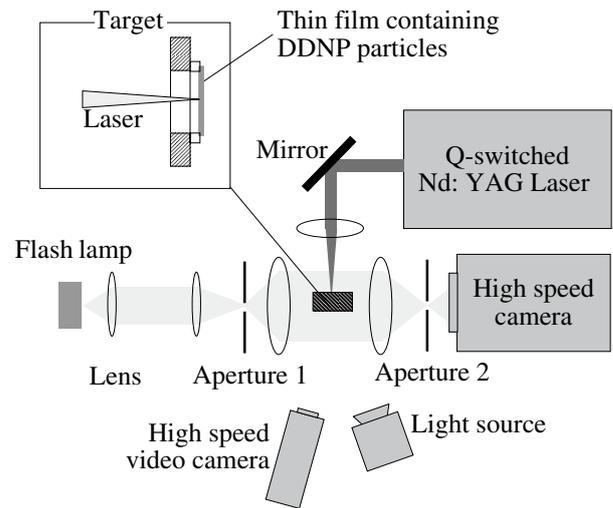
Fig. 3 Optical setup for high-speed photography with high-speed camera and video camera. Both camera systems can be used simultaneously for selected experimental conditions.
