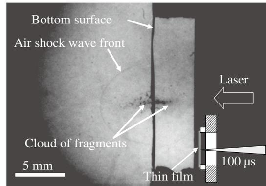
**Fig. 5** High speed photographic records of monolayer DDNP / CTA reactive film combustion process. Film specifications are as follows: DDNP / CTA = 8 / 2, and have  $33 \mu\text{m}$  in thickness prepared by PAD method. Pulse laser fluence is  $29 \text{ J cm}^{-2}$ . Delay time is  $10 \mu\text{s}$ .
