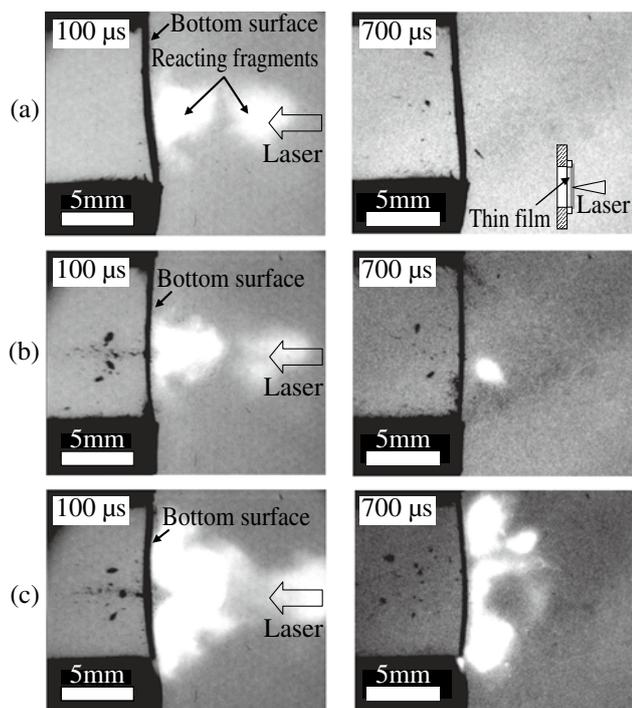
Fig. 10 High speed photographic records of the combustion process of multi-layered DDNP / CTA reactive film with different mass ratios. Film thickness for all cases is 250  $\mu\text{m}$ . Mass ratio DDNP / CTA is 8 : 2 for cases (a), and 9 : 1 for cases (b) and (c), respectively. Laser fluence is 15  $\text{J cm}^{-2}$  for cases (a) and (b), and 30  $\text{J cm}^{-2}$  for case (c), respectively.
