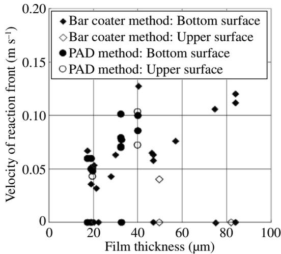
**Fig. 9** Reaction front velocity of monolayer DDNP / CTA reactive thin film whose thickness is less than 100  $\mu\text{m}$ . Mass ratio DDNP / CTA is 8 : 2. Laser fluence for all the data is 29-30  $\text{J cm}^{-2}$ . Data of zero velocity stands for no combustion.
