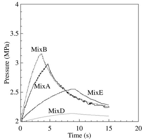
Fig. 2 Pressure-time history of 5-ATZ / oxidizer mixtures from closed vessel test.
