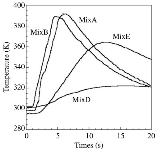
Fig. 3 Temperature-time history of 5-ATZ / oxidizer mixtures from closed vessel test.
