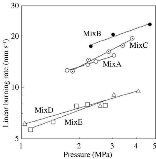
Fig. 1 Linear burning rate of 5-ATZ / oxidizer mixtures.
