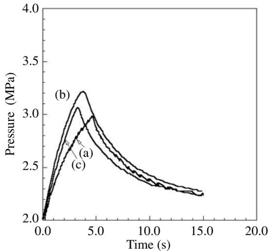
Fig. 5 Effect of the particle size on the pressure-time history of 5-ATZ / LiClO<sub>4</sub> mixtures from closed vessel test.
