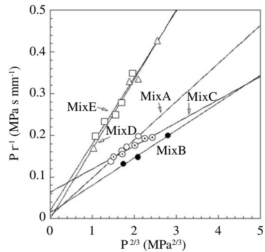
Fig. 4 GDF correlation of linear burning rate with:  $(P/r) = a + b P^{2/3}$
