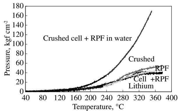
Fig. 3 Pressure vs. temperature curves of the lithium cells mixing with RPF in the MCPVT.
