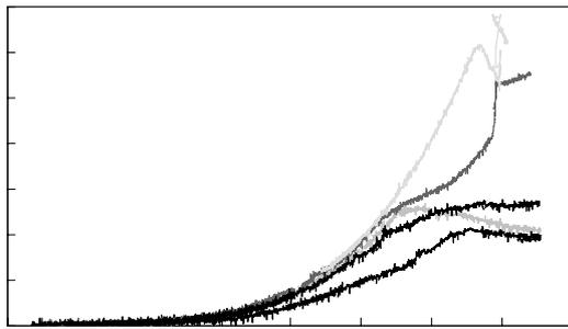
Fig. 2 Pressure vs. temperature curves of the lithium cells and mixture with water in the MCPVT.
