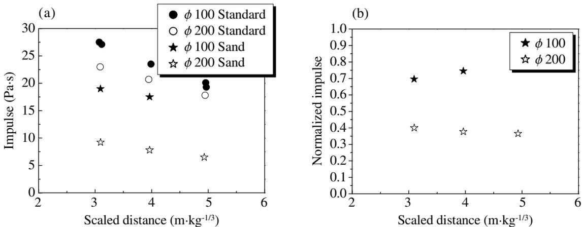
Fig. 3 (a) Relation between the positive impulse and the scaled distance from the charge.
