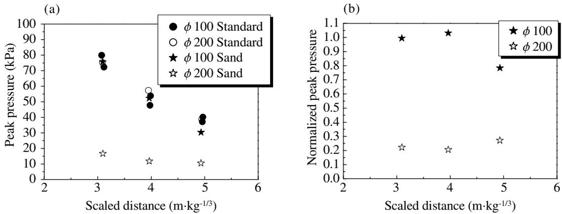
Fig. 2 (a) Relation between the peak pressure and the scaled distance from the charge.
