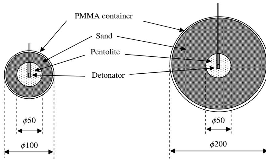
Fig. 1 Sectional view of the spherical containers, filled with the pentolite and the sand.
