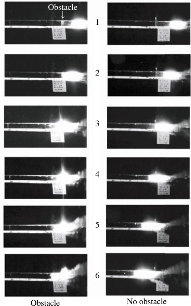
Fig. 3 PAS progression in PMMA tube.
