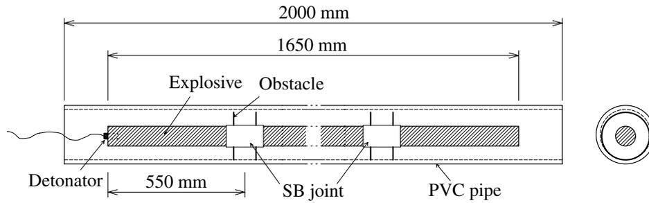
Fig. 2 Experimental arrangement used in test series B.
