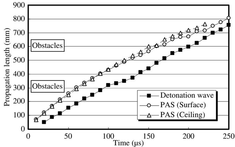
Fig. 6 Propagation length of detonation wave and PAS.
