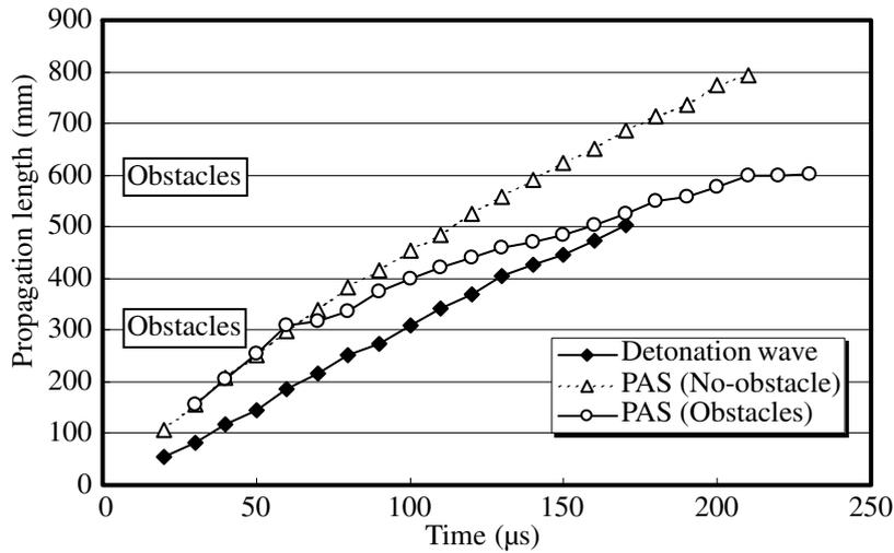
Fig. 4 Propagation length of detonation wave and PAS (Deco ; 2.0).
