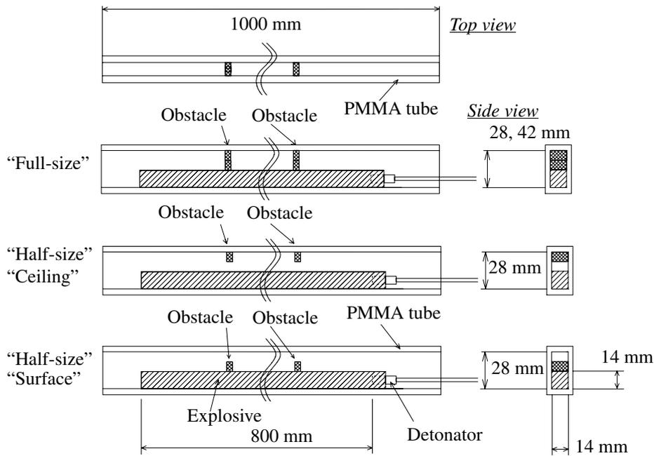
Fig. 1 Experimental arrangement used in test series A.
