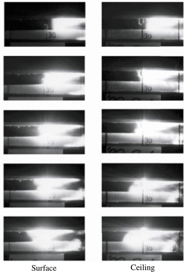
Fig. 5 PAS progression in PMMA tube.
