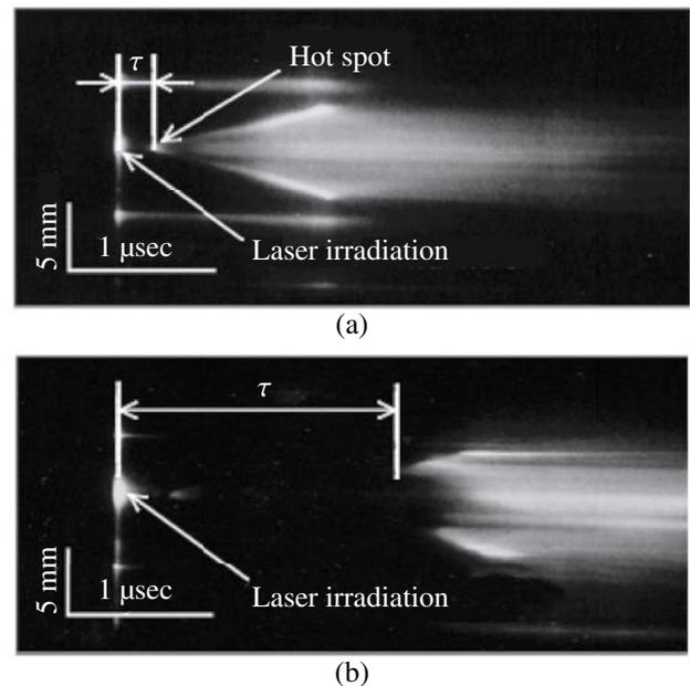
Fig. 5 Streak photograph of light emission associated with detonation of PETN powder by pulse laser ablation of ground glass plate. Diffusion plate of #400 was used. Laser fluence is set to (a)  $15.1 \text{ J cm}^{-2}$ , and (b)  $9.1 \text{ J cm}^{-2}$ , respectively. Initiation delay time  $\tau$  is defined as in the figure.
