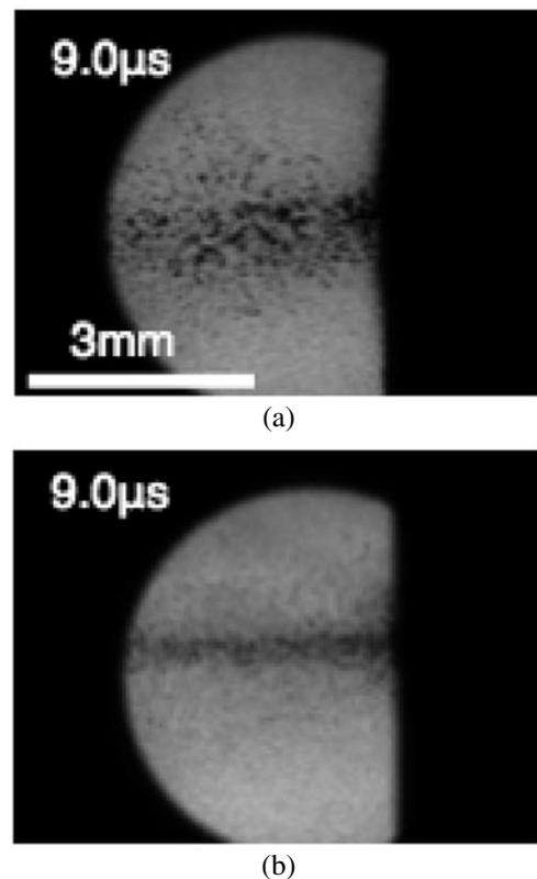
Fig. 2 High speed camera photos of laser ablation of optical diffusion plate at later delay time of  $9.0 \mu\text{s}$ . Two examples of diffusion plates with different surface roughness, #240 (photo (a)) and #800 (photo (b)). Laser energy, focused diameter and fluence is  $0.38 \text{ J}$ ,  $1.4 \text{ mm}$ , and  $25 \text{ J cm}^{-2}$ , respectively.
