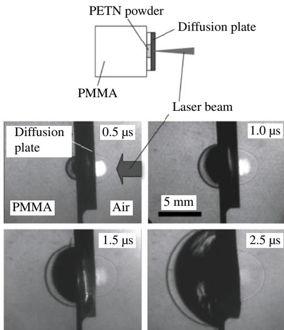
Fig. 4 High speed photograph of stress waves in PMMA attached to PETN powder induced by the detonation of PETN powder for the diffusion plate with surface roughness #800.
