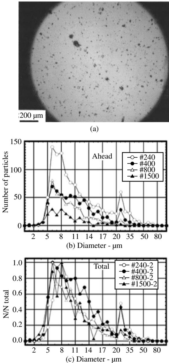
Fig. 3 Particle size distribution for each diffusion plate with different surface roughness. Figure (b) corresponds to size distribution for particles both at PMMA plate ahead of and beneath the target. Figure (c) shows particle size distribution for particles normalized by the peak value, respectively.
