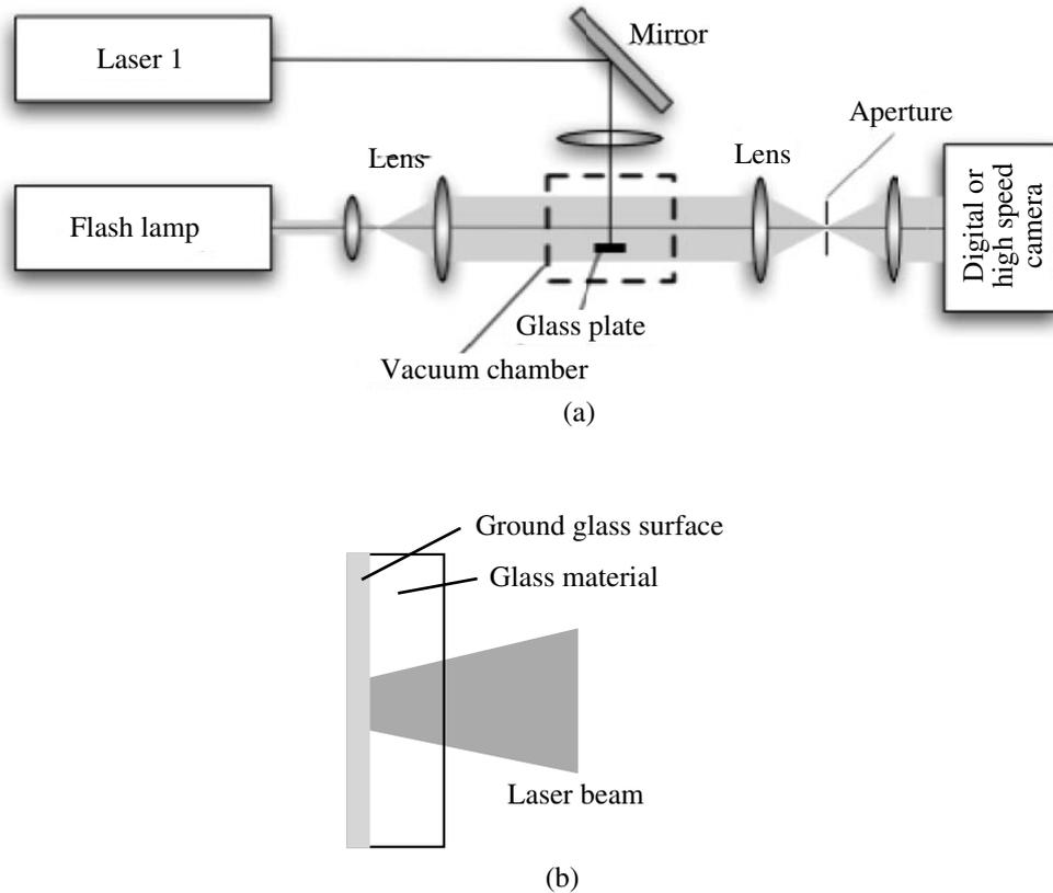
Fig. 1 Optical setup for laser shadowgraph or high speed framing camera observation. Vacuum chamber is installed only for ablation in vacuum experiments.
